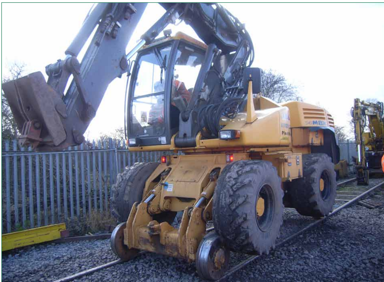
Figure 2: Example Type 9B high ride RRV with traction and braking through the road wheels to the rail wheels
