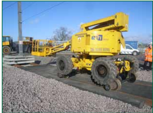
High ride self-propelled boom RRV
