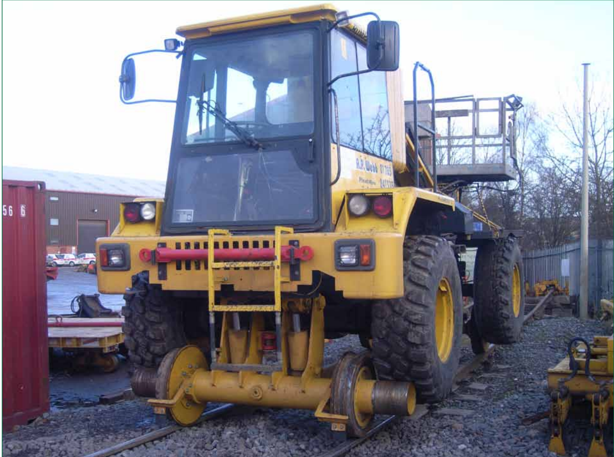
Figure 4: Type 9B high ride RRV with extensions fitted to the rail wheels (spigots)
