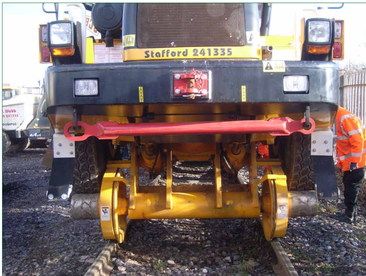
Figure 5: Road wheel/spigot contact area
