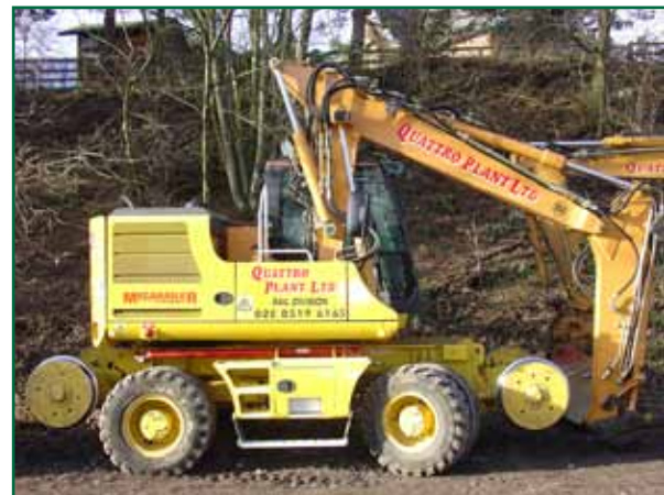
High ride wheeled excavator RRV
