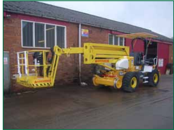
High ride dumper with access platform RRV
