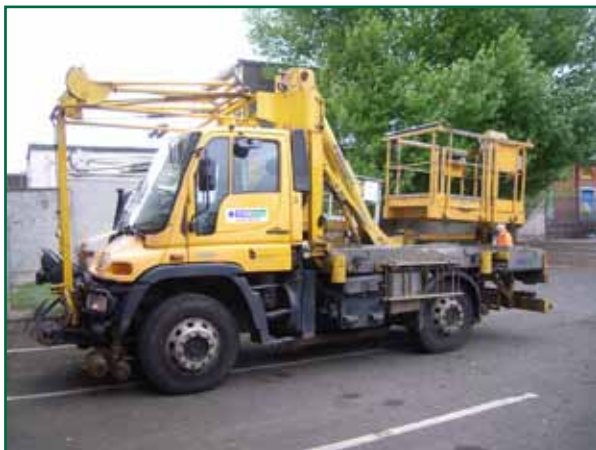
Low ride Unimog with access platform RRV
