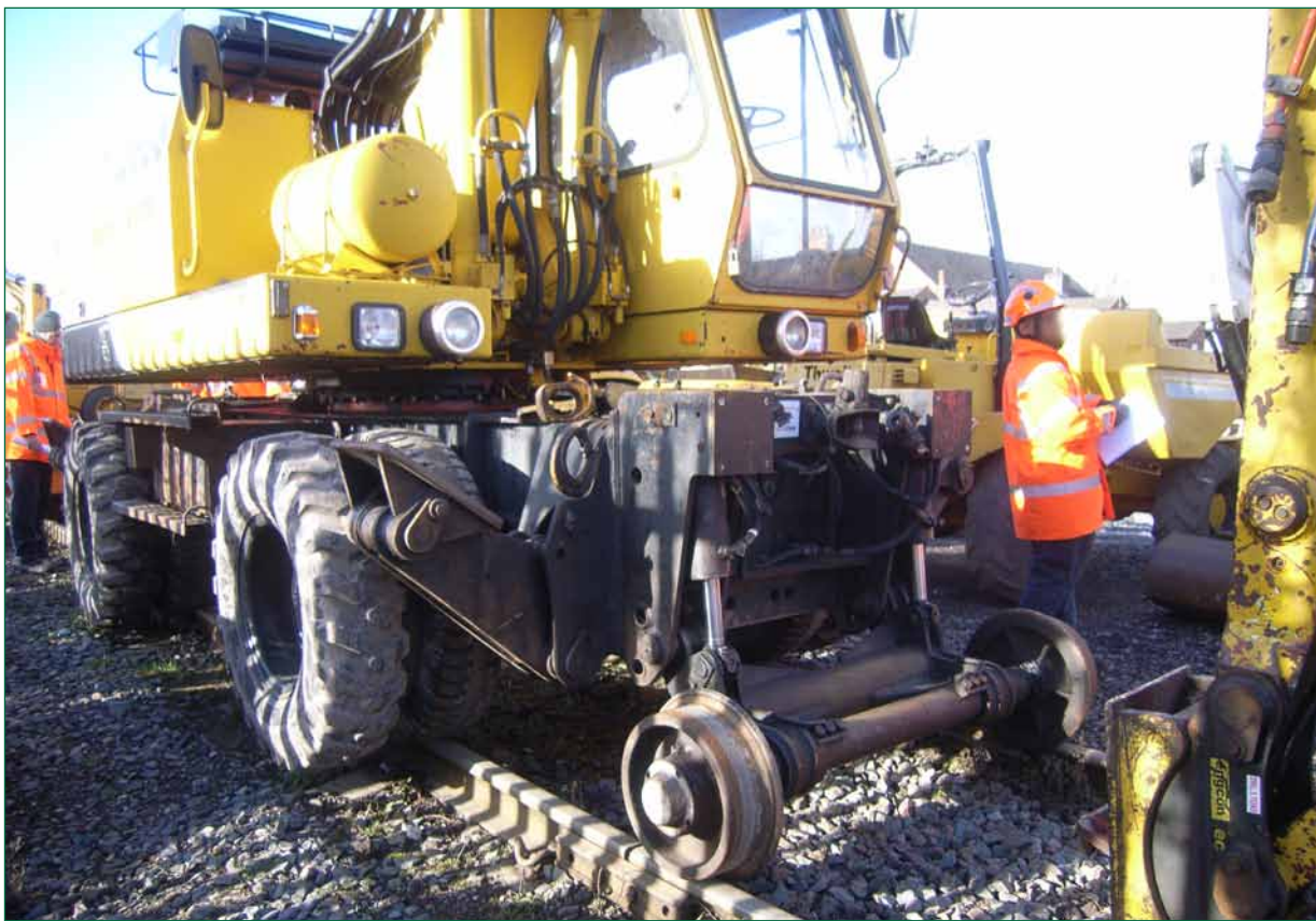
Figure 3: Example Type 9C low ride RRV with traction and braking through the road wheels
