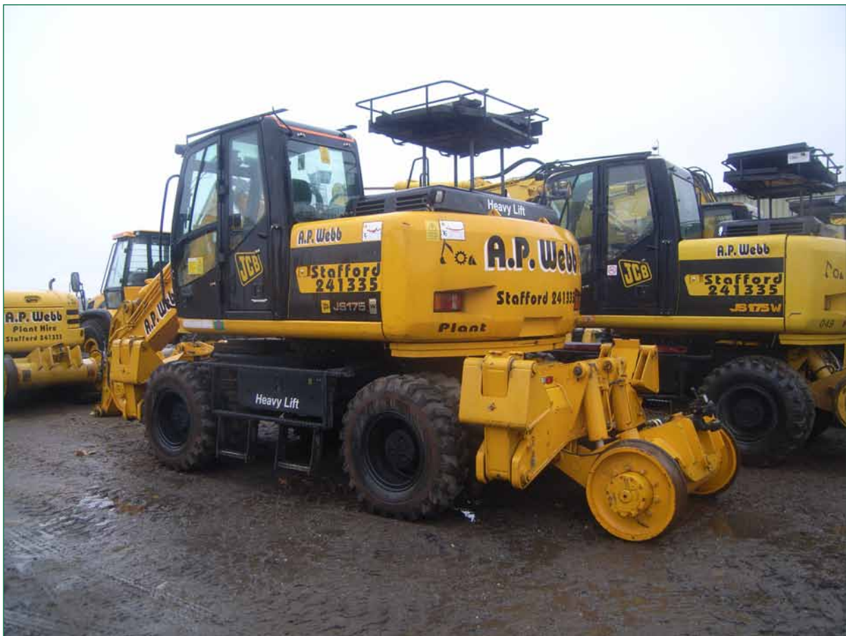
Figure 1: Example Type 9A RRV with self-powered rail wheels
