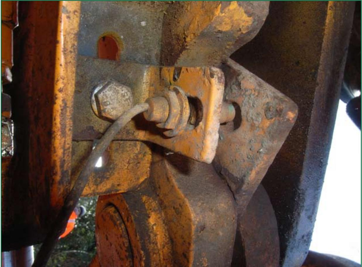
Figure 6: The sensor for detecting that the rail wheels are fully deployed
