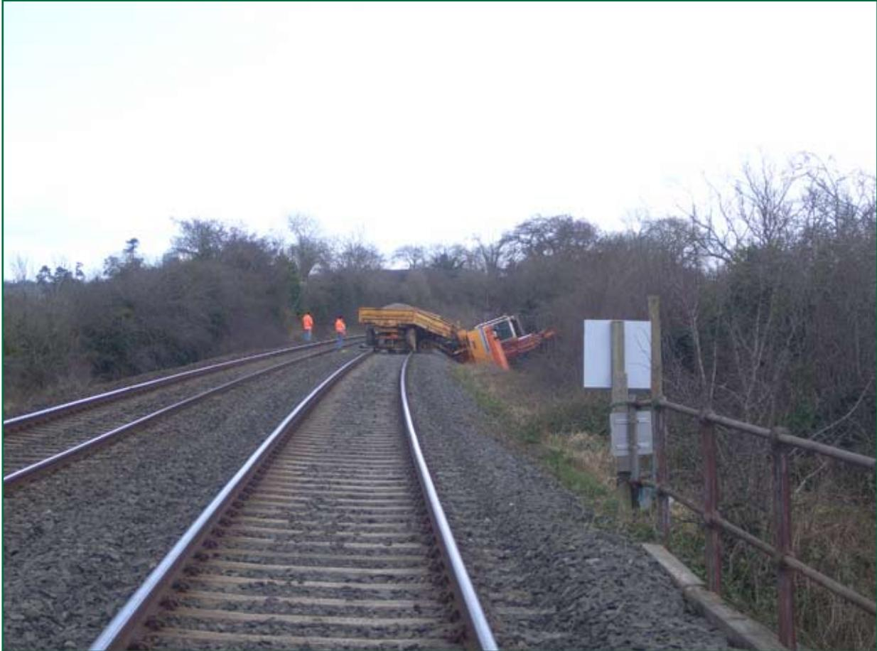
Figure 3: The track is curved, canted (banked), and on a rising gradient in the direction of travel
