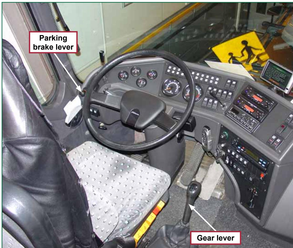
Figure 7: The layout of the Bova Futra's driving position showing parking brake and gear lever
