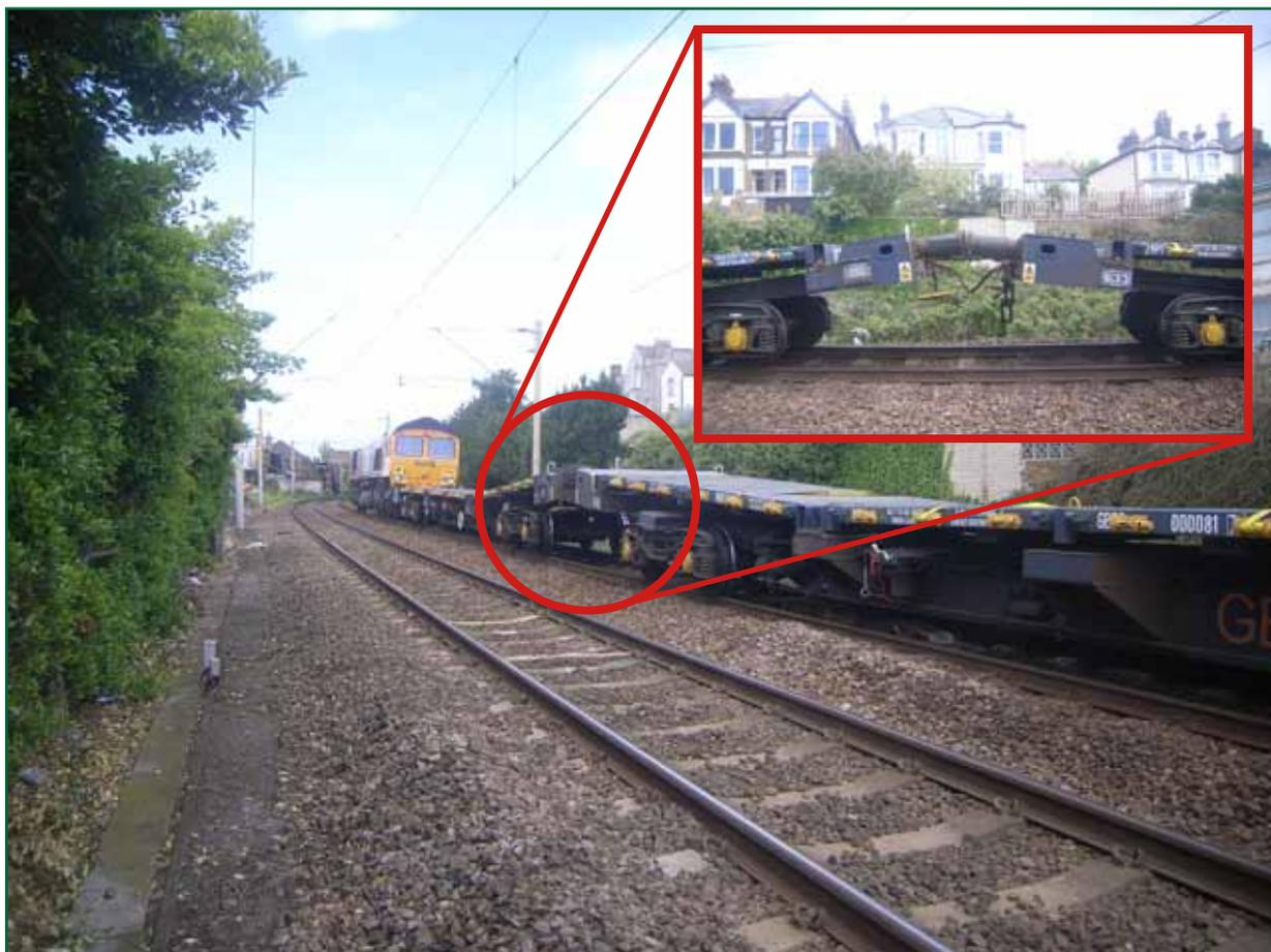
Figure 9: Photograph and (inset photograph) of train 6T64 and FEA wagon damage sustained as a result of the collision
