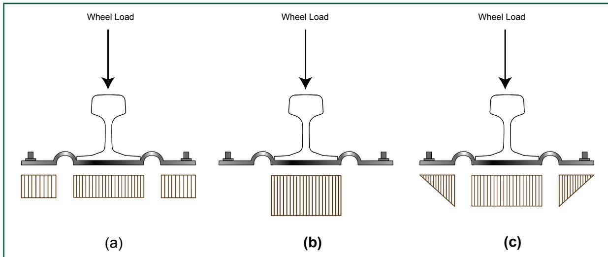
Figure 6: Pressure distributions beneath baseplate
