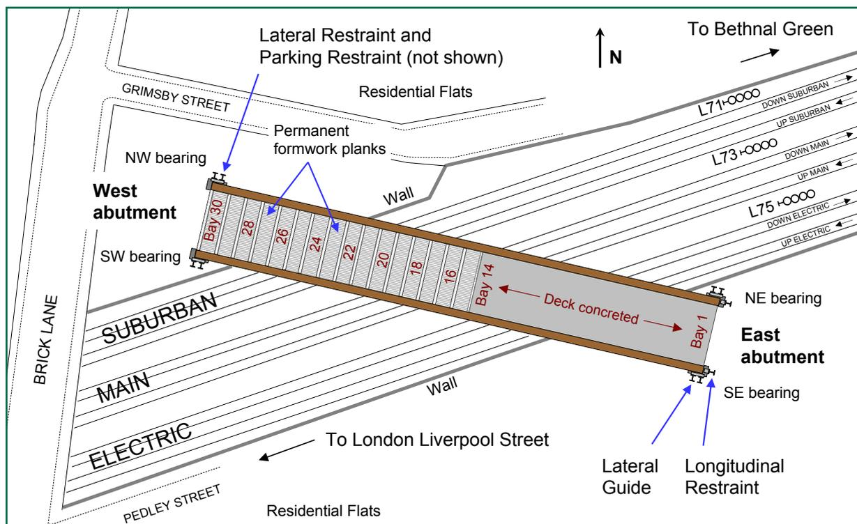
Figure 3: Schematic diagram of bridge in position, showing main construction features at time of partial collapse
