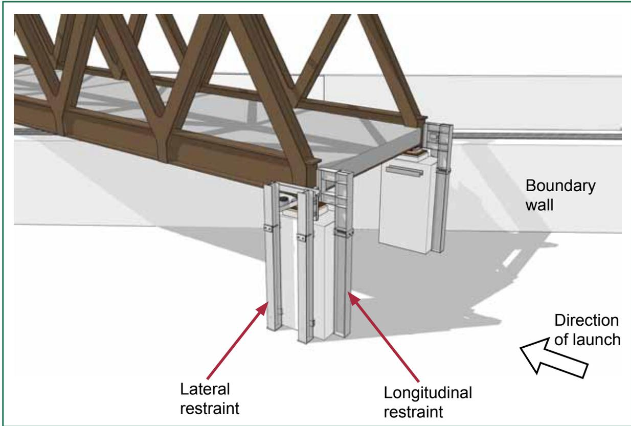
Figure 19: Schematic diagram showing temporary works at the east abutment following erection of the longitudinal restraints.
