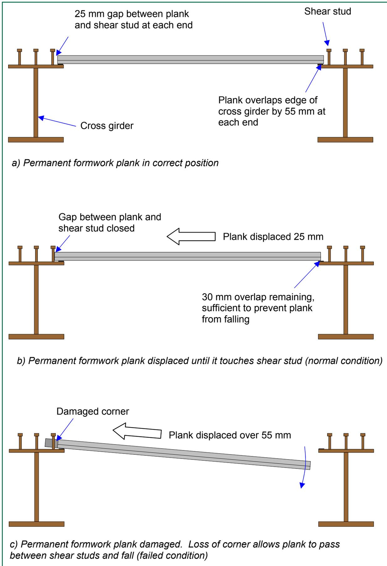
Figure 26: Schematic diagram showing effect of shear stud in restraining movement of a permanent formwork plank.
