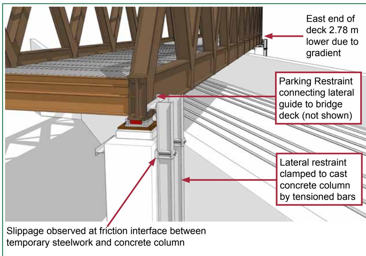
Figure 18: Schematic diagram showing location of parking restraint at the west abutment, acting as a temporary fixed bearing.
