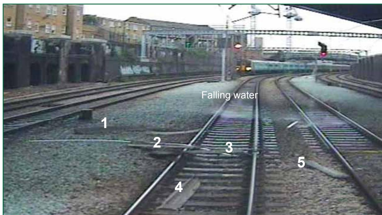
Figure 5: Image from CCTV equipment on train 1K12 showing debris on track immediately before the collision. The position of the five pre-cast concrete permanent formwork planks is indicated
