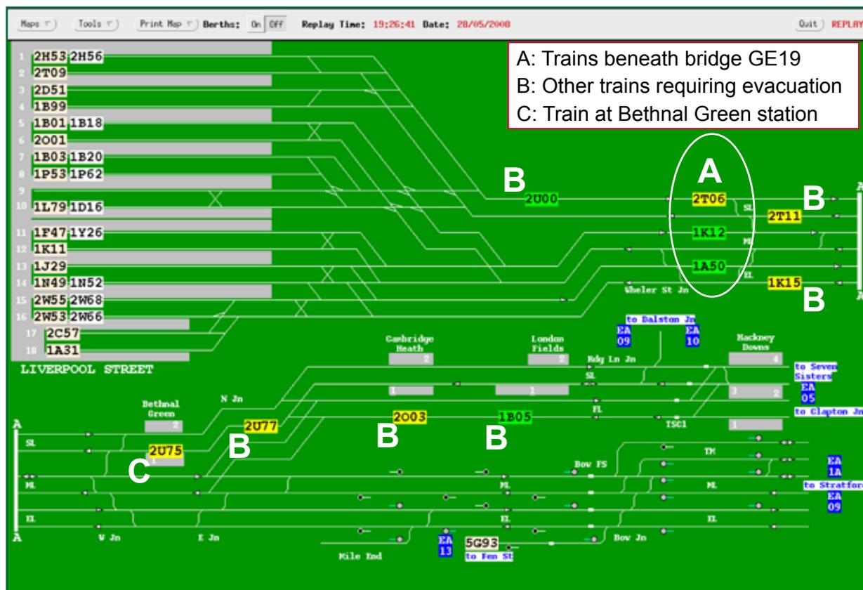
Figure 9: Image of signalling data at 19:26 hrs showing location of stationary trains following accident.
