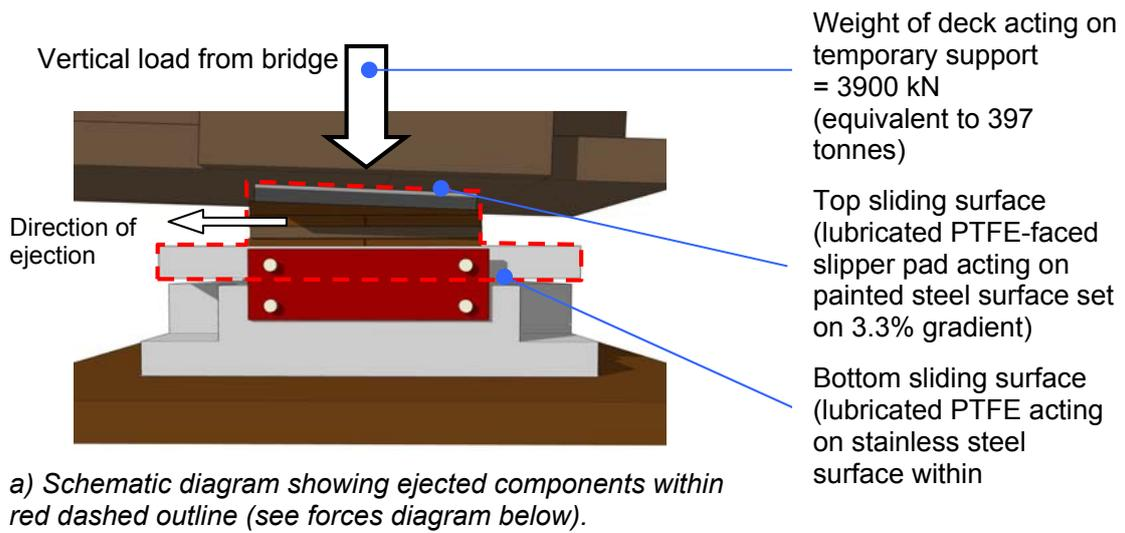
The load from the bridge deck acting on the top sliding surface ( $N$ ) can be separated into vertical and horizontal components,  $N_v$  and  $N_h$ , where  $N_h$  is the horizontal component acting to destabilise the temporary support.
