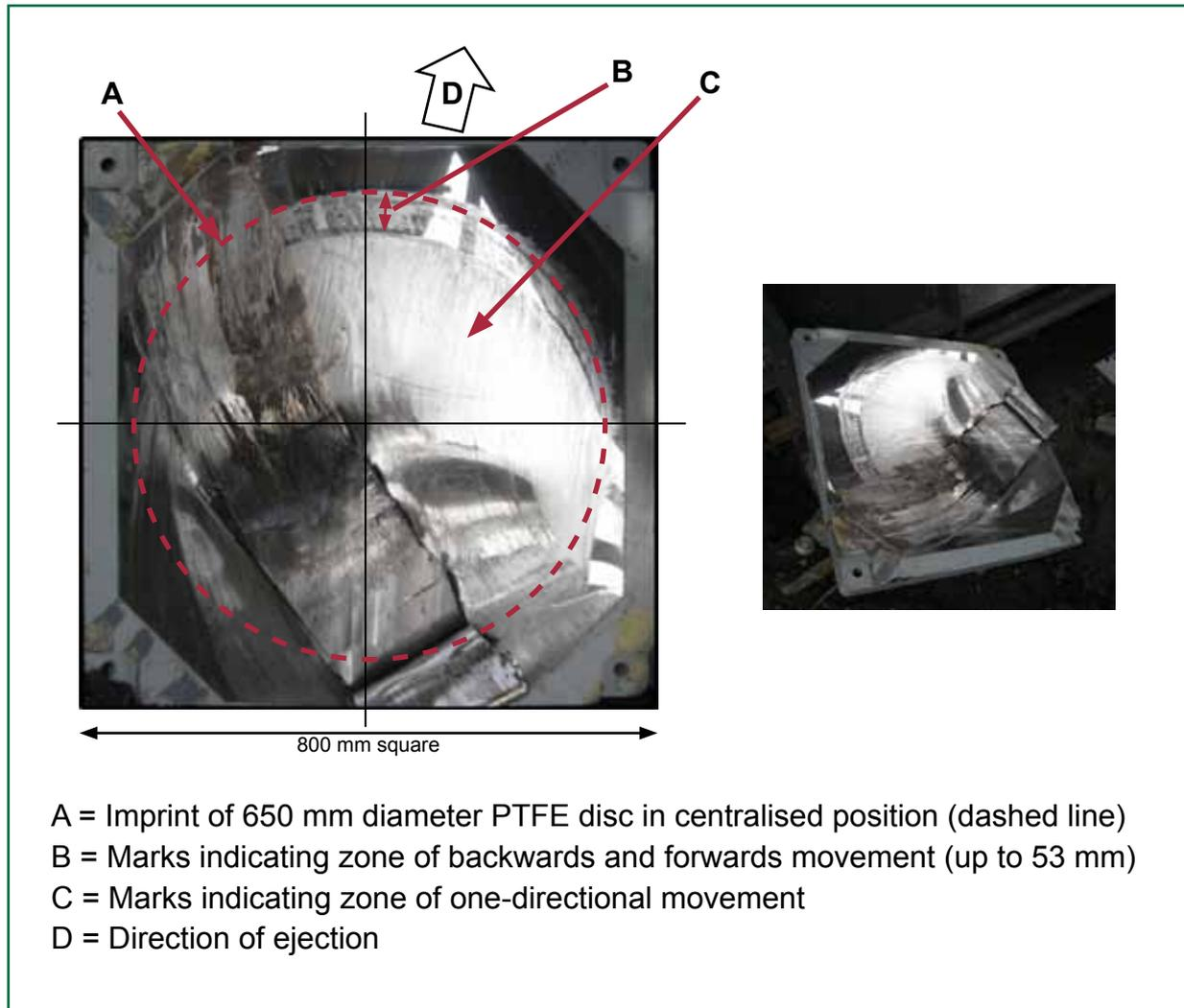
Figure 24: re-orientated photograph of the underside of the south-east bearing top plate, showing major dimensions and (inset) as-found.
