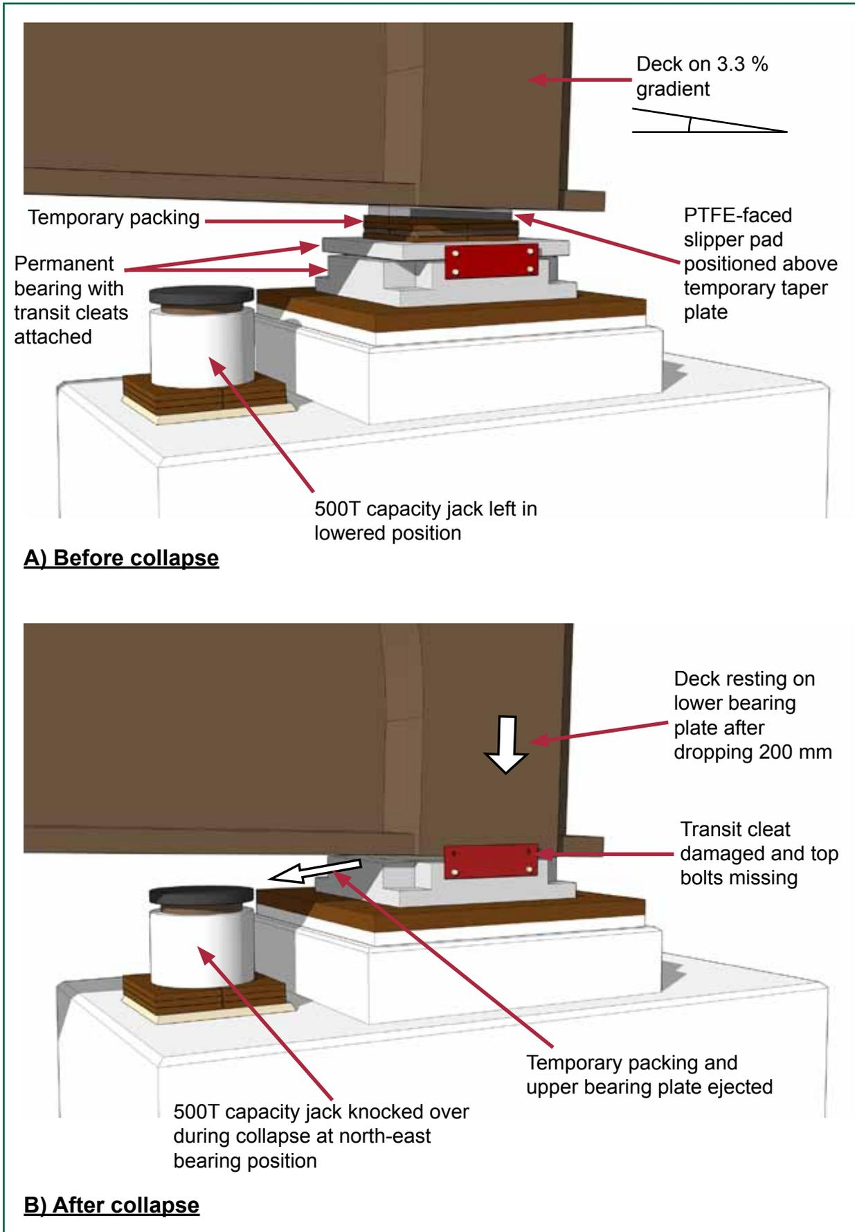
Figure 21: Schematic diagrams of south-east bearing and temporary support before and after collapse
