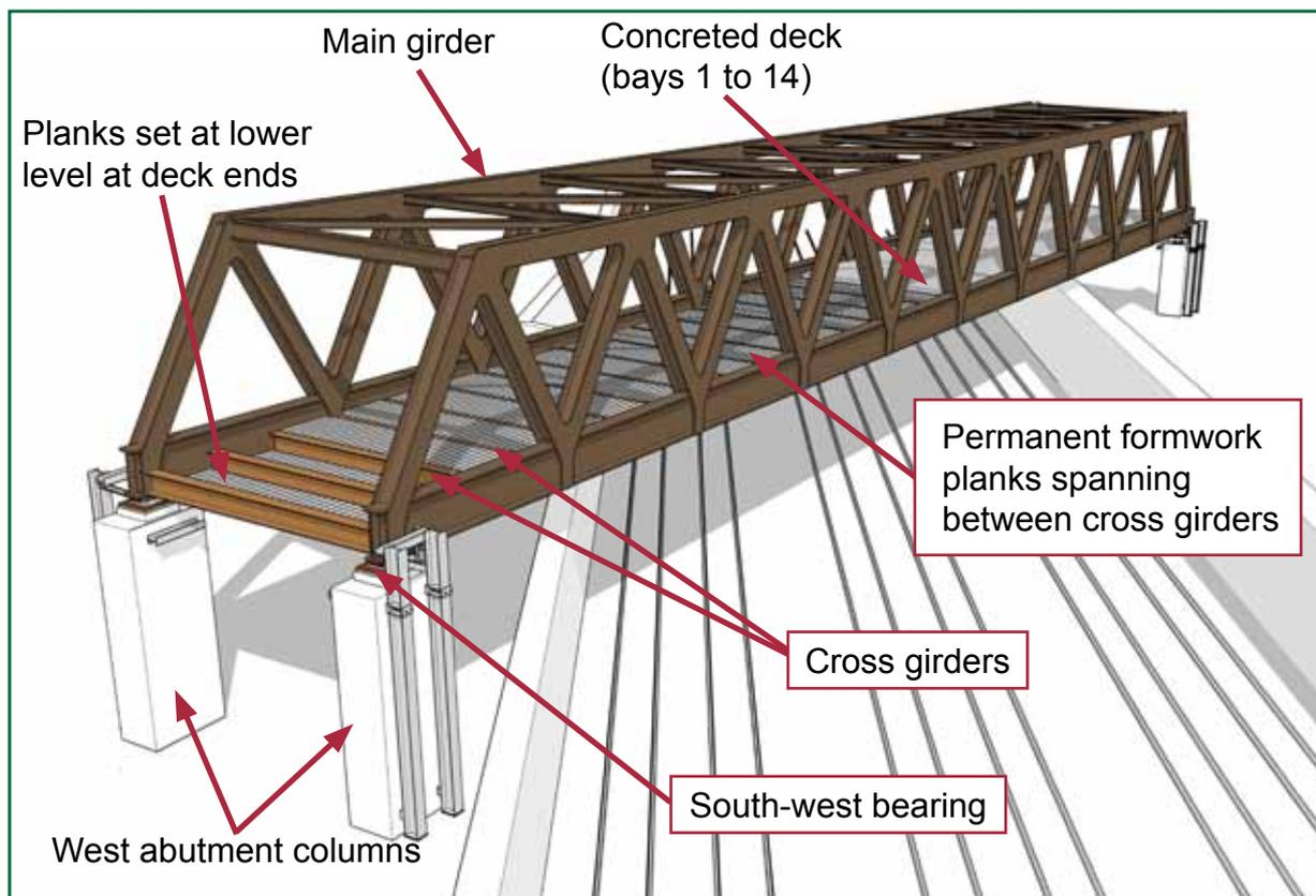
Figure 14: Schematic diagram showing main deck components
