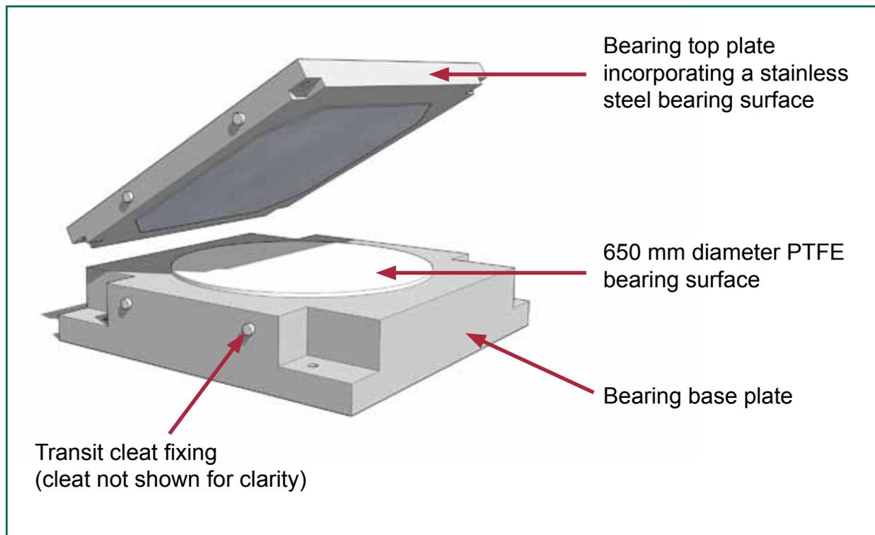
Figure 13: Schematic diagram showing top and base plates of a free permanent bearing
