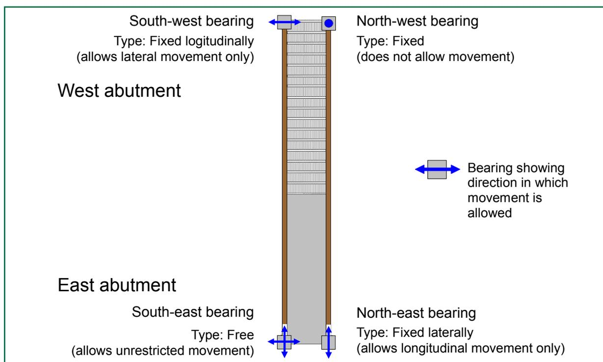
Figure 12: Bearing, showing direction in which movement is permitted
