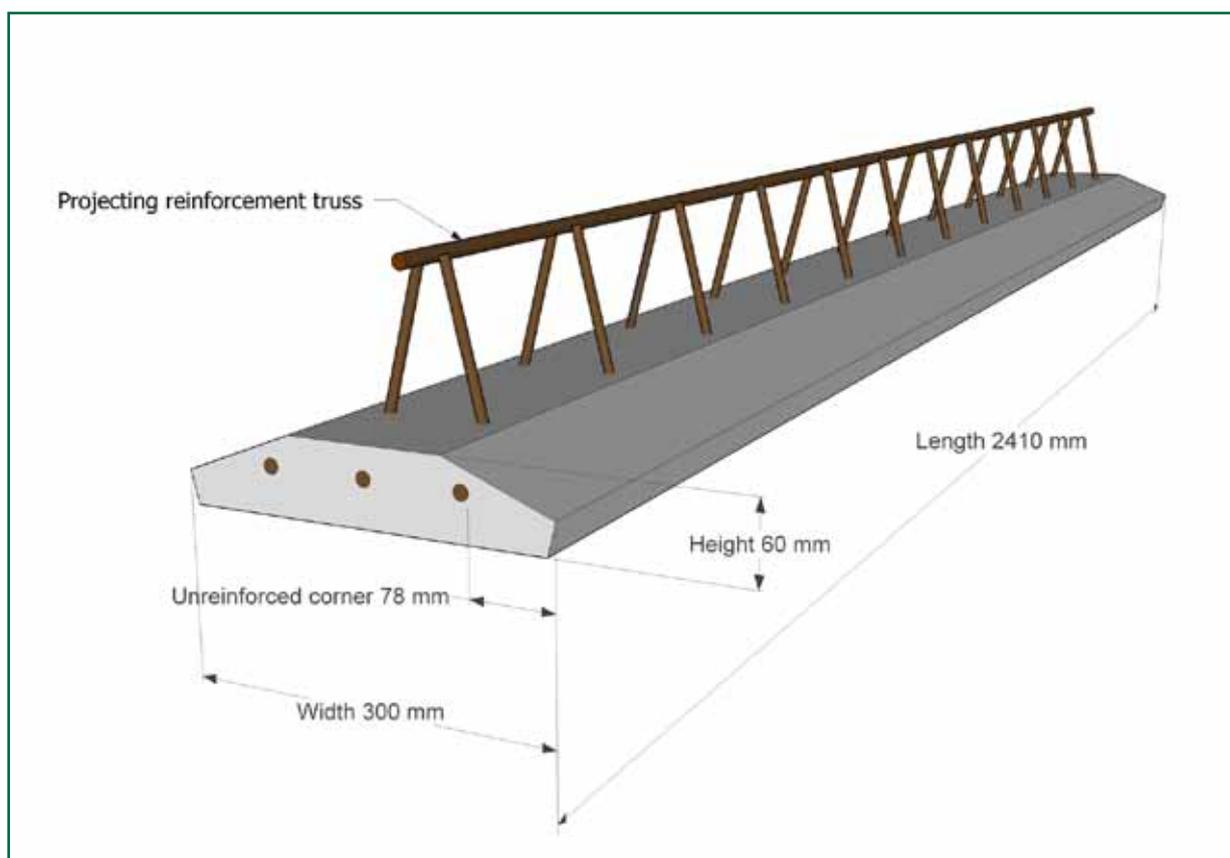
Figure 15: Schematic diagram of a permanent formwork plank installed on bridge GE19.
