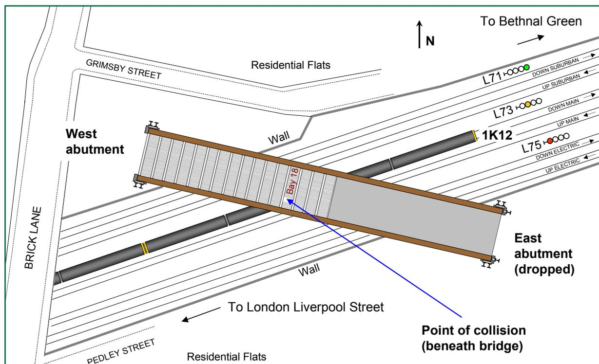
Figure 7: Situation at 19:18 hrs with train 1K12 stopped partly beneath bridge GE19
