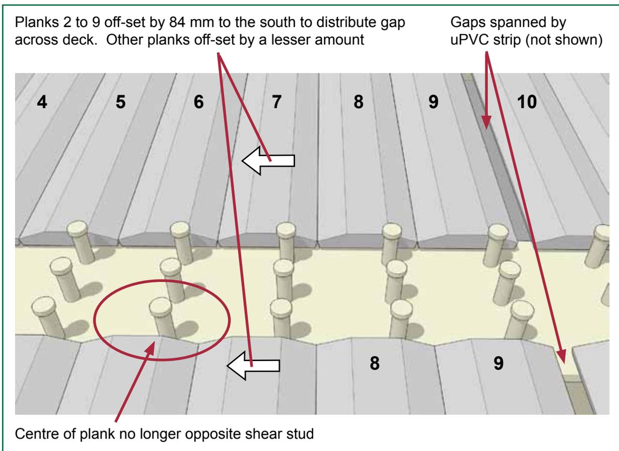
Figure 17: Schematic diagram showing a typical deck bay, and the modified relationship between shear studs and permanent formwork planks.
