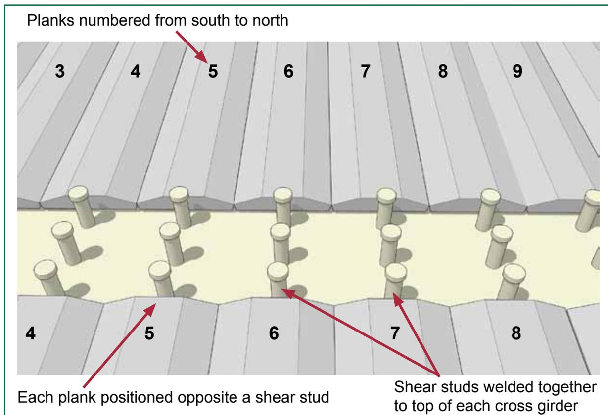
Figure 16: Schematic diagram showing a typical deck bay, and the as-designed relationship between shear studs and permanent formwork planks
