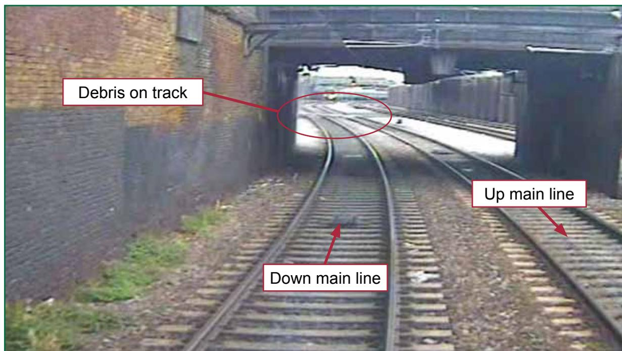
Figure 4: Image from CCTV equipment fitted to train 1K12, six seconds before collision with debris
