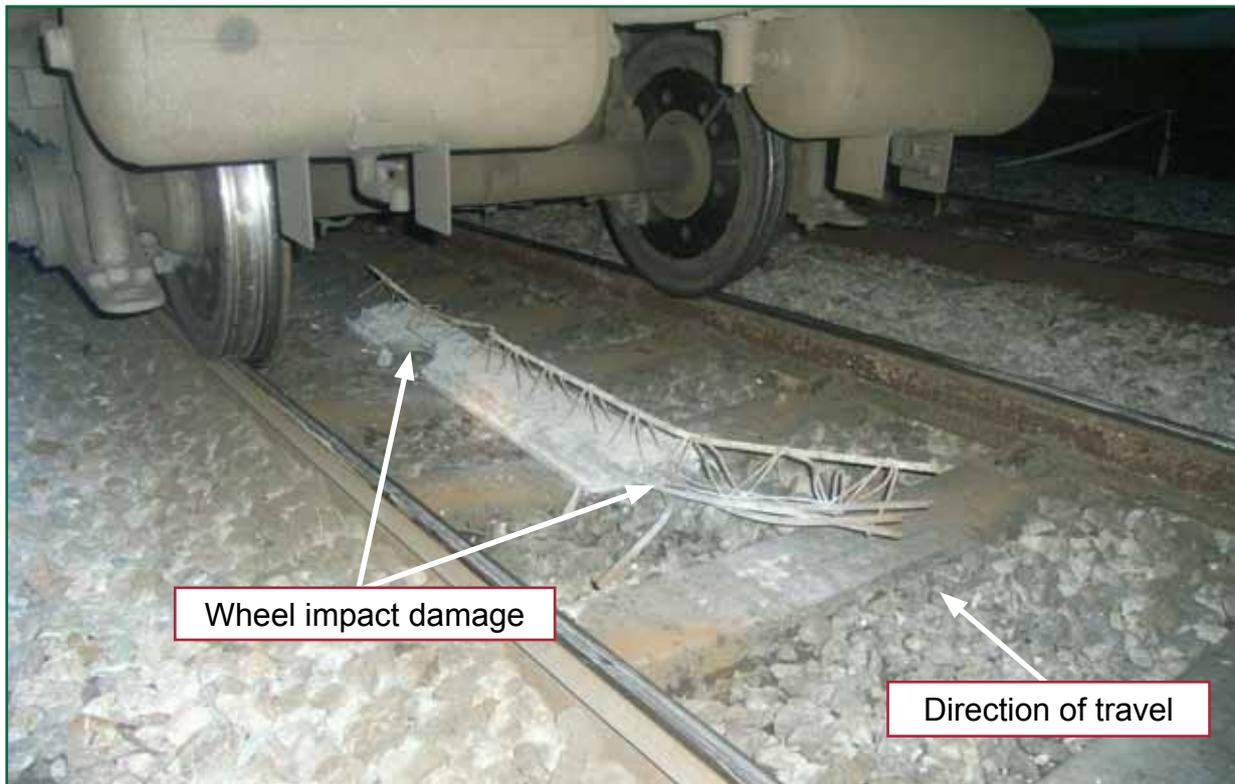
Figure 6: Damaged permanent formwork plank after being dragged forwards under train 1K12
