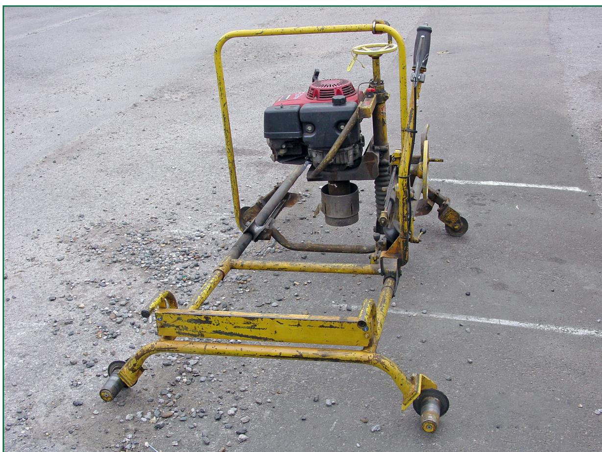
Figure 3: NV3 track grinding machine
