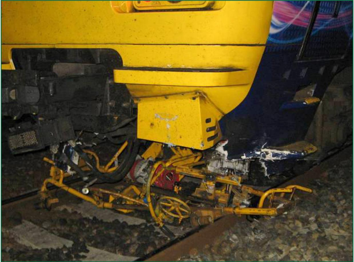
Figure 4: The train with the grinding equipment underneath (photograph courtesy of Network Rail)
