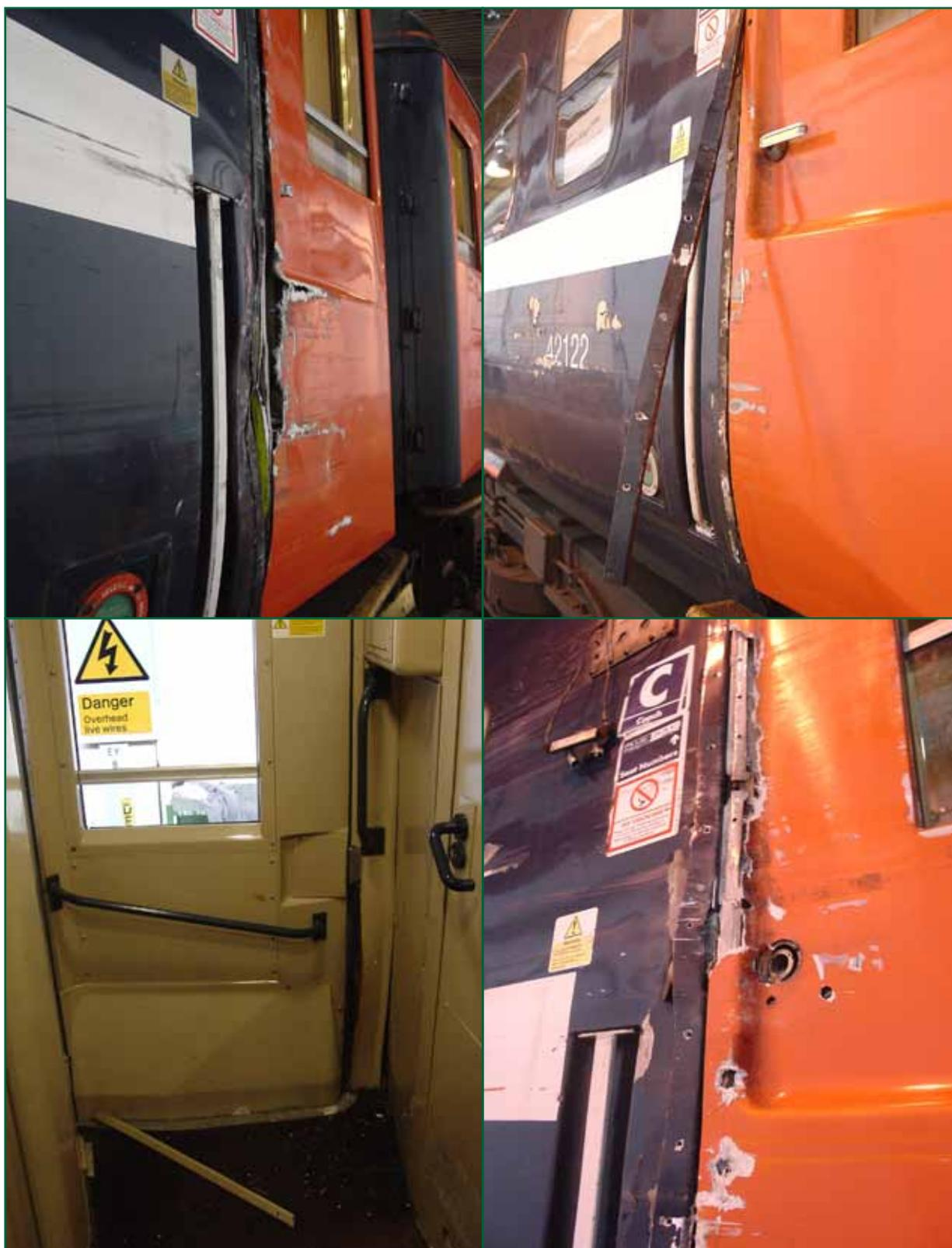
Figure 7: Examples of damage to right-hand side of southbound train 1A16
