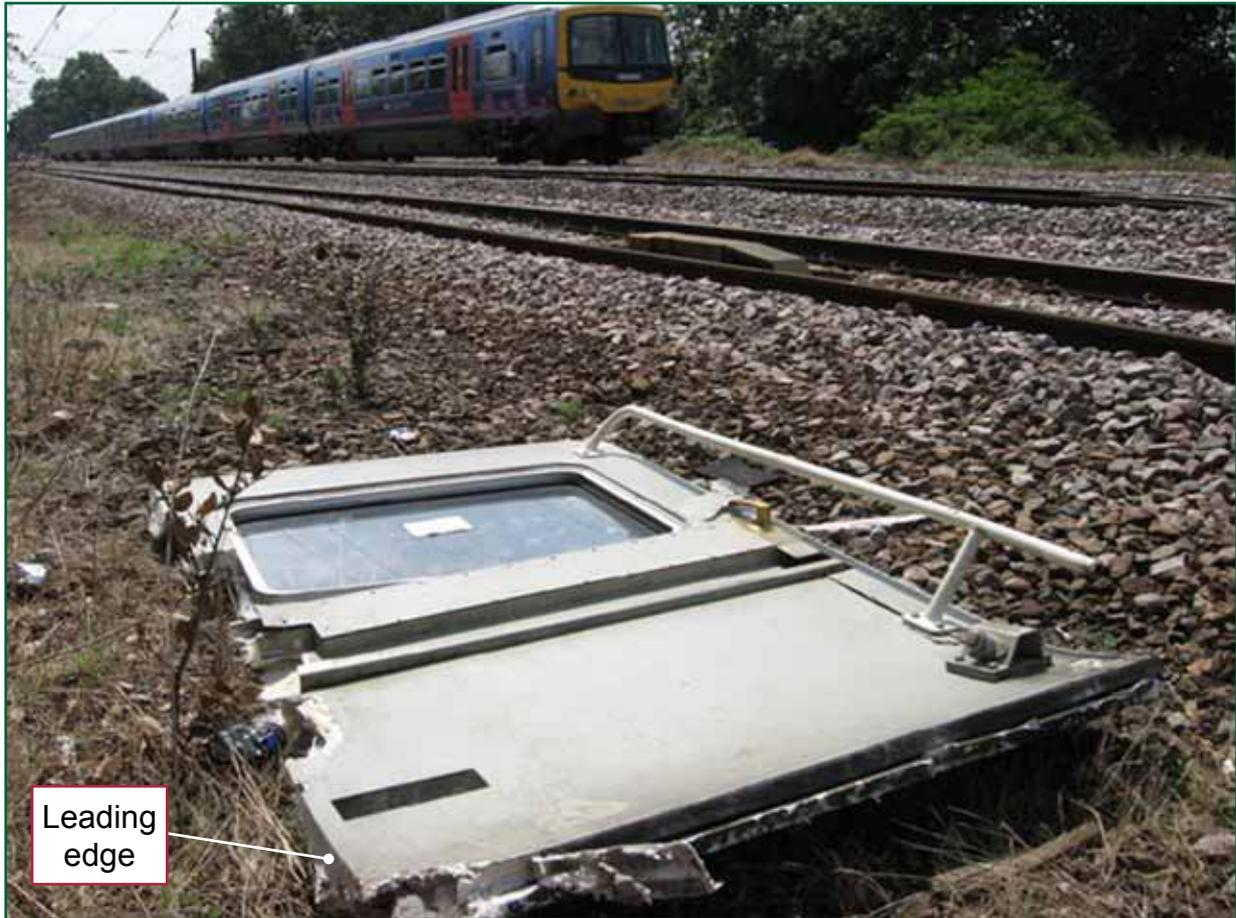
Figure 3: The door involved in the incident as found (the train shown is not related to the incident)
