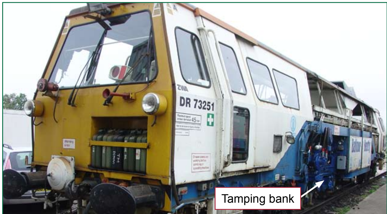
Figure 1: Plasser 07 series tamping machine showing position of the tamping banks
