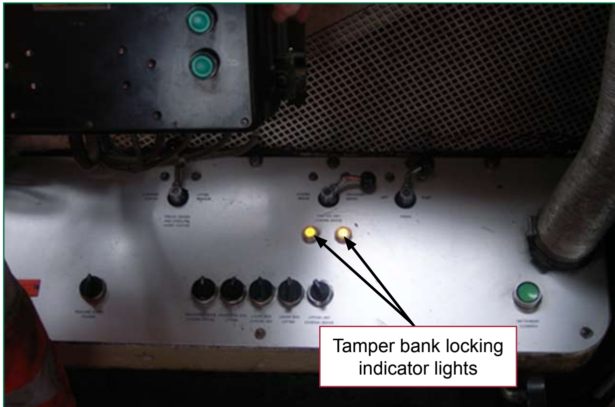
Figure 3: Tamper bank locking indicator lights
