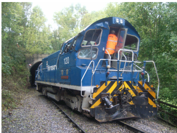
Figure 3: collision damage to derailed locomotive
