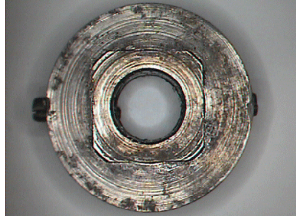
Figure 8: Top view of collar showing parts of fractured pin
