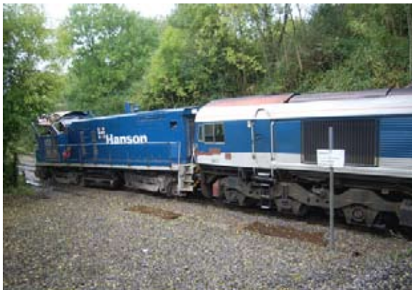
Figure 1: derailed shunting locomotive and mainline locomotive
