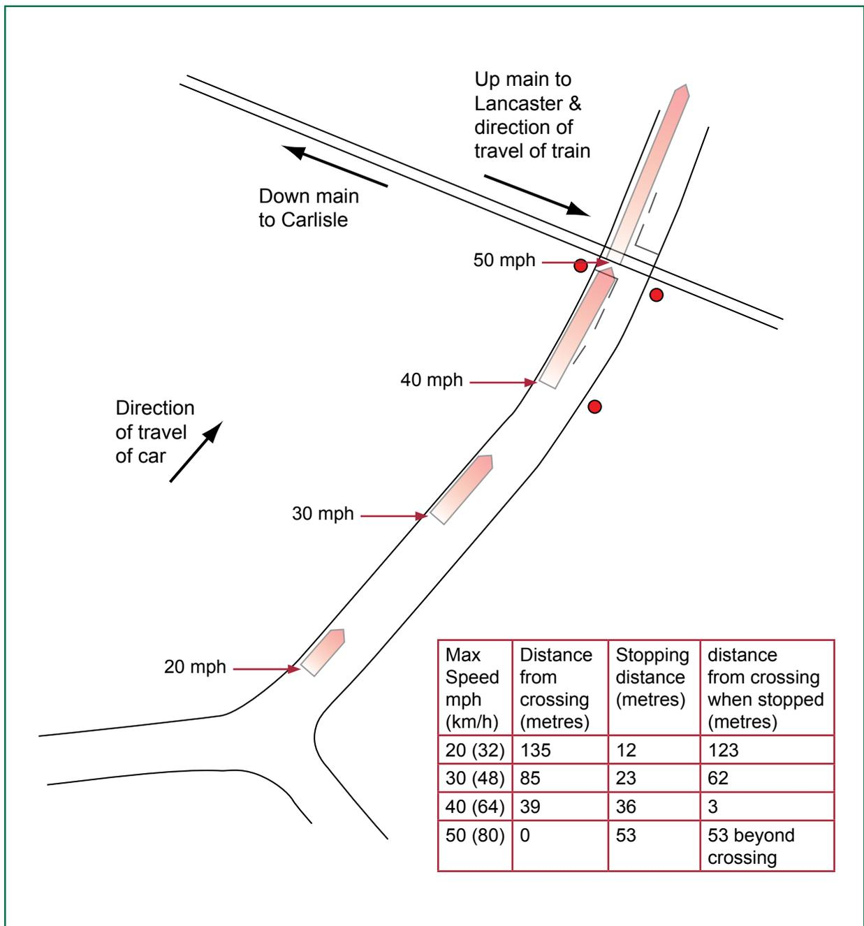
Figure 13: Stopping distances from maximum safe speed on the approach to Wraysholme crossing
