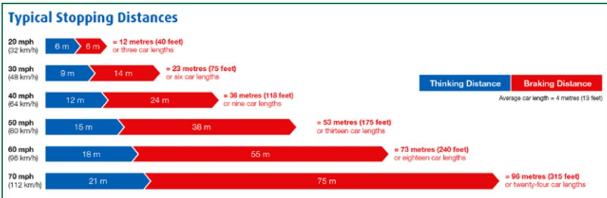
Figure 12: Stopping distances extracted from the Highway Code
