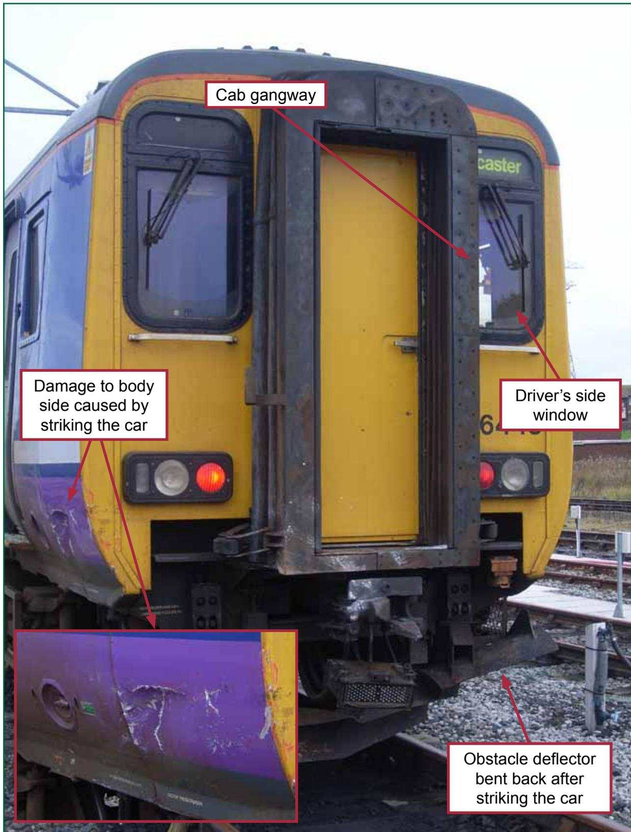
Figure 8: The train and its leading cab
