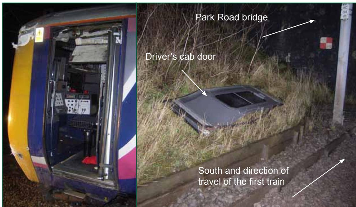
Figure 12: Damage to the southbound train
