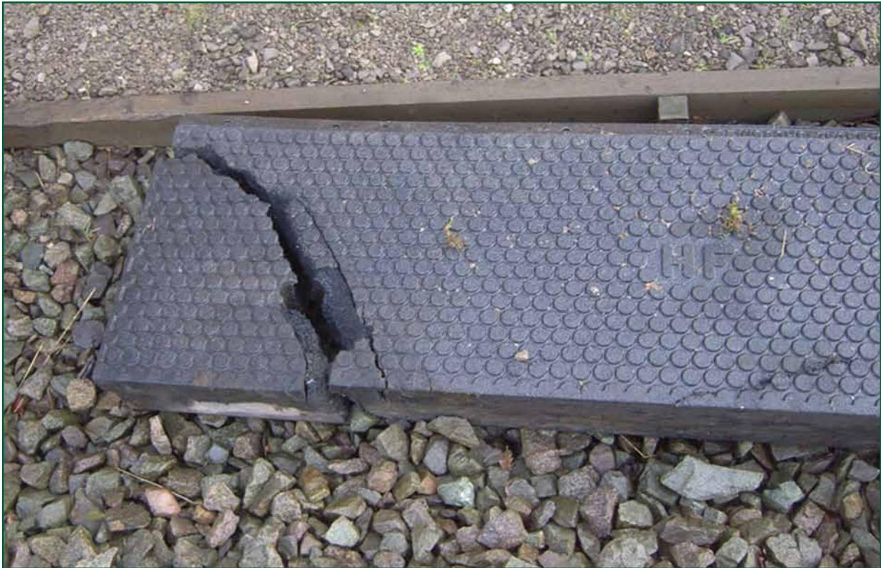
Figure 14: The rubber block damaged by the northbound train (the pieces were placed together for the image)
