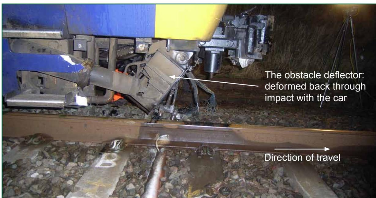
Figure 8: Damage to the southbound train caused by striking the car
