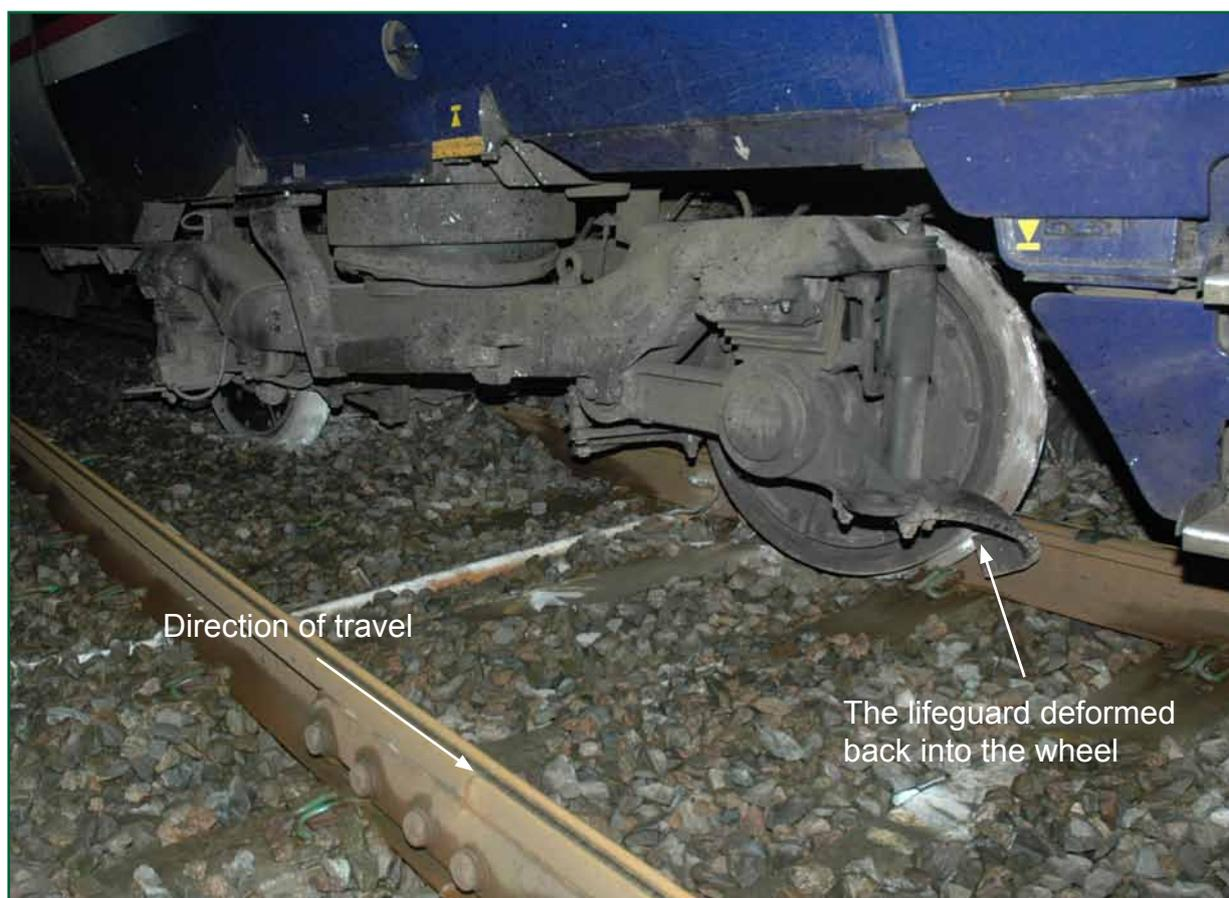
Figure 9: The leading right-hand wheel, bearing against the left-hand rail (photograph courtesy of British Transport Police)
