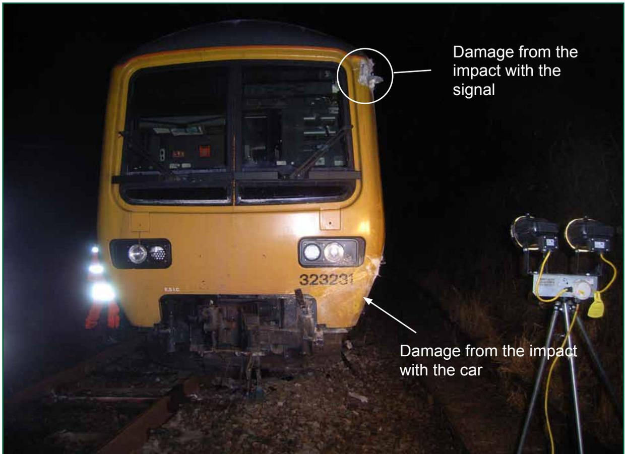
Figure 11: The driving cab of the southbound train
