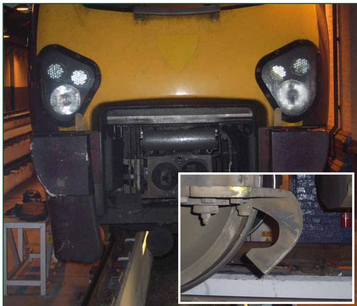
Figure 13: The driving cab of the northbound train and (inset) damage to the right-hand lifeguard
