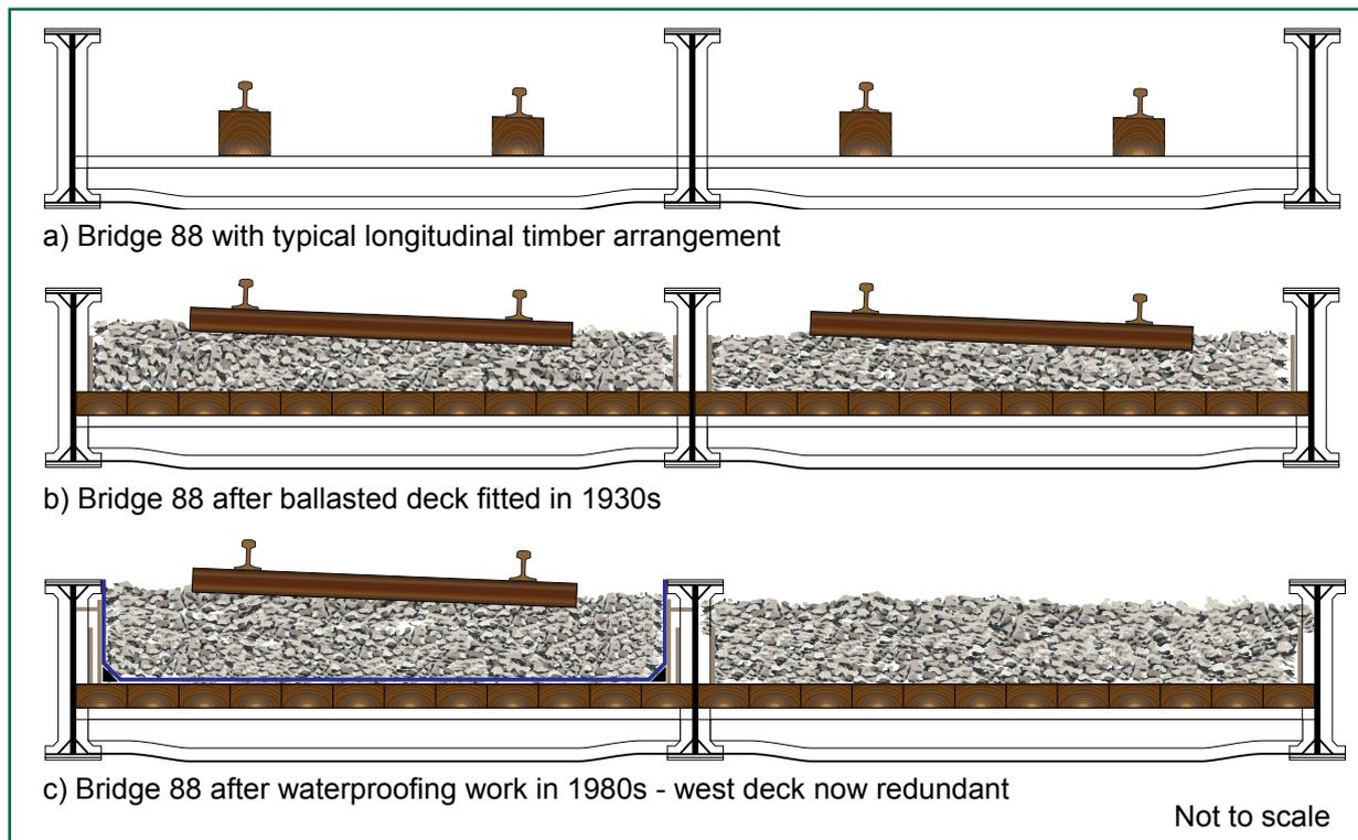
Figure 7: Cross-section of the deck of Bridge 88 showing the modifications made since it was constructed
