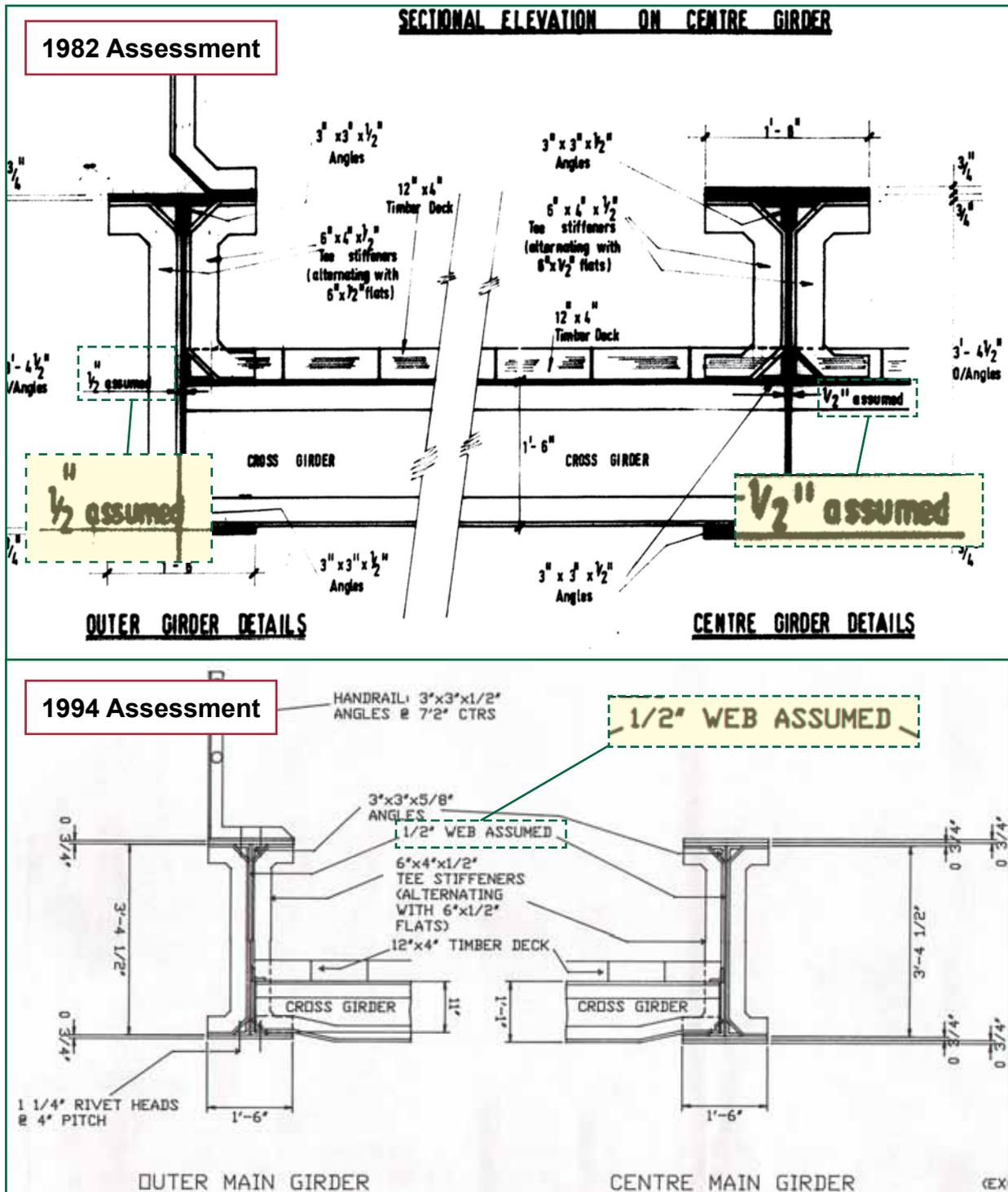
Figure 20: Extracts from the drawings prepared for the 1982 and 1994 Assessments showing the cross-section of the main girders (images courtesy of Network Rail)
