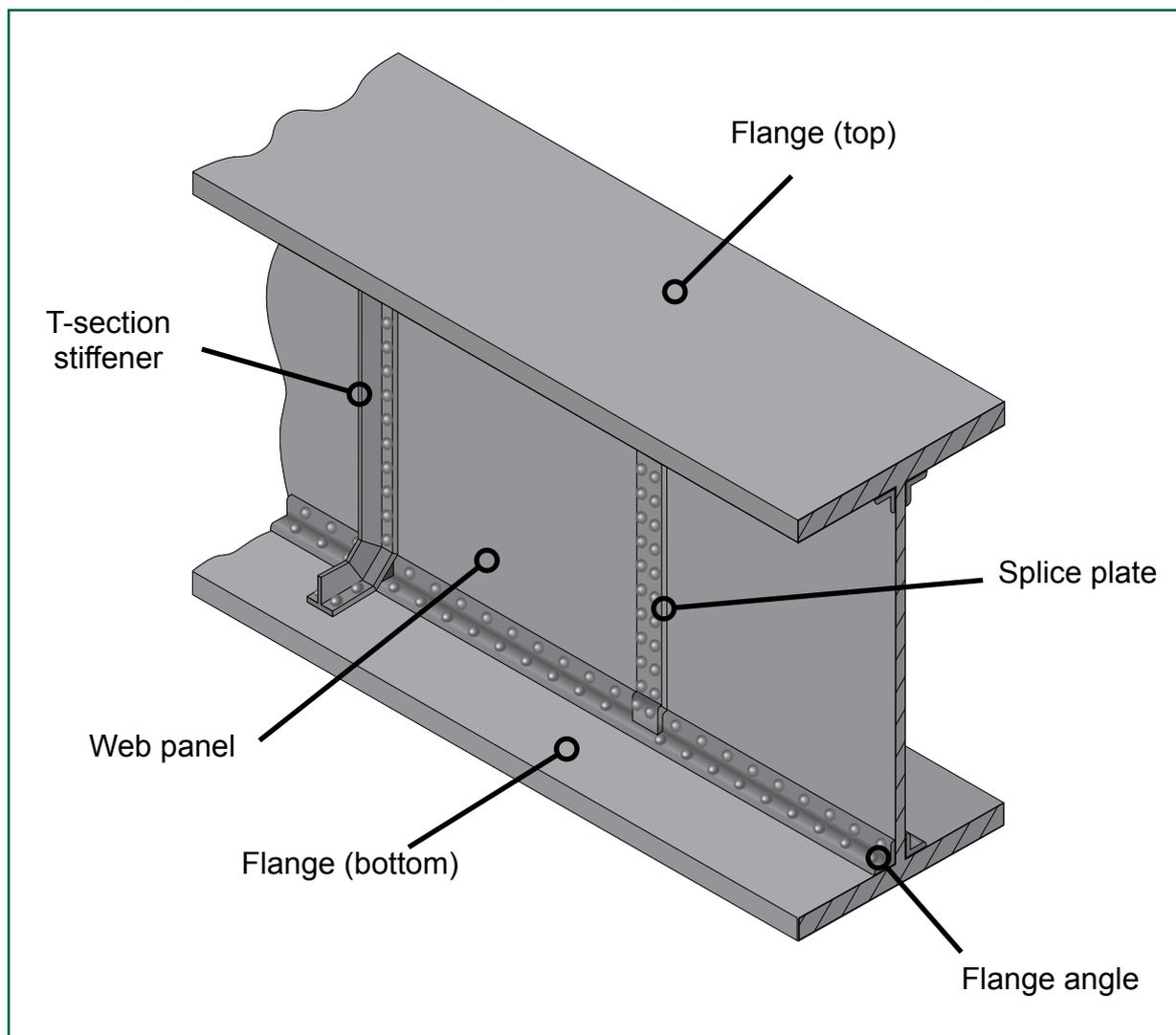
Figure E1: Diagram showing a typical main girder web panel and associated parts
