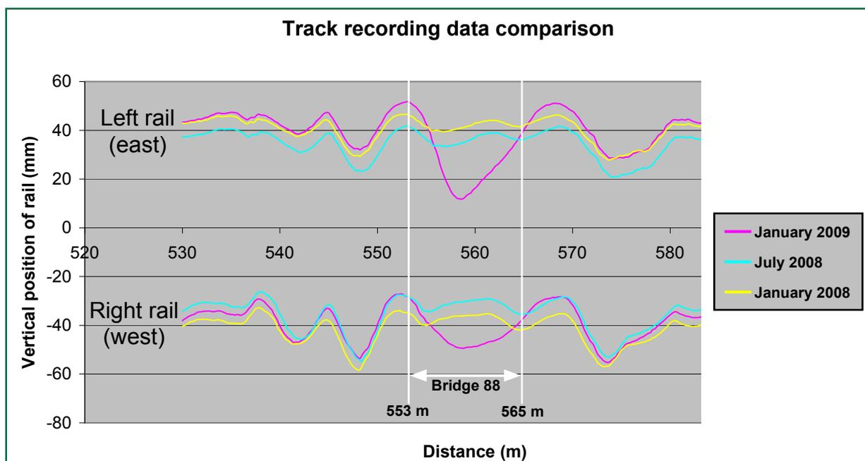
Figure 13: Vertical geometry of the track measured in the vicinity of Bridge 88
