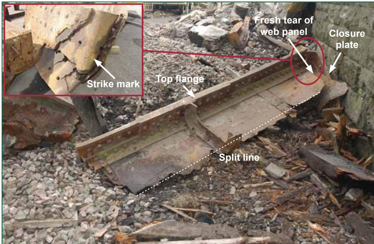
Figure 12: Upper part of the south end of the centre main girder showing the horizontal split line, the folded closure plate and fractured flanges (main photograph courtesy of British Transport Police)
