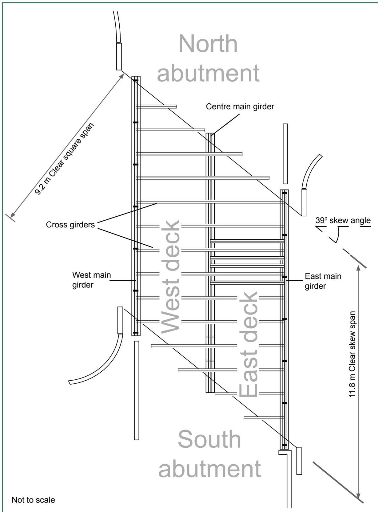
Figure 5: Plan view of Bridge 88 superstructure
