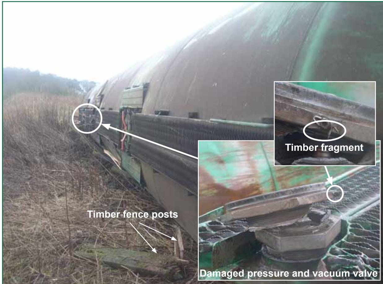
Figure 24: Damaged pressure and vacuum valve on wagon 7
