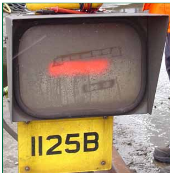
Figure 9c: 1125B point position indicator displaying a red bar
