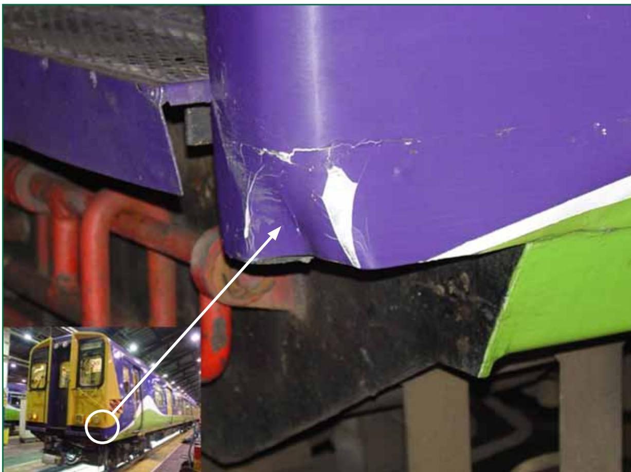
Figure 5: Damage to the front of unit 313119
