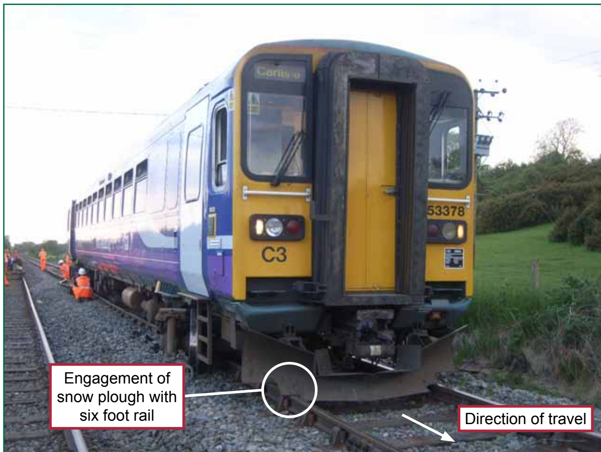
Figure 5: Leading end of unit 153378, showing positions of right-hand wheels and engagement of snow plough with right-hand rail
