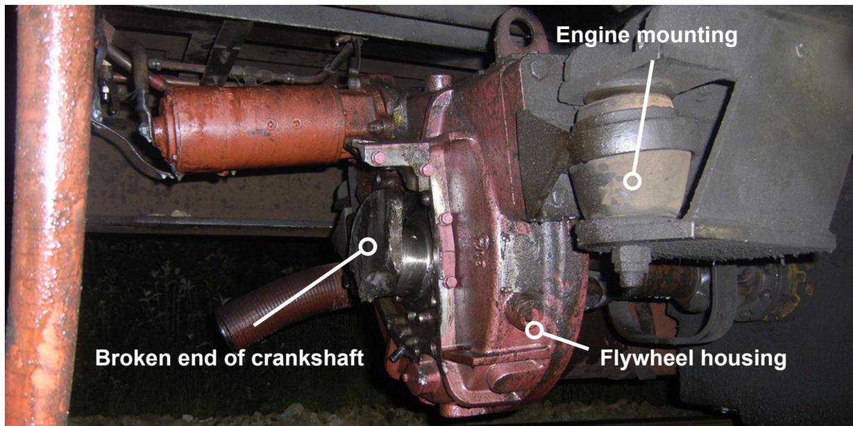
Figure 2: Flywheel housing and engine mounting points
