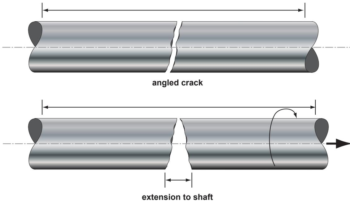
Figure 4: Diagram showing how fracture lengthened crankshaft
