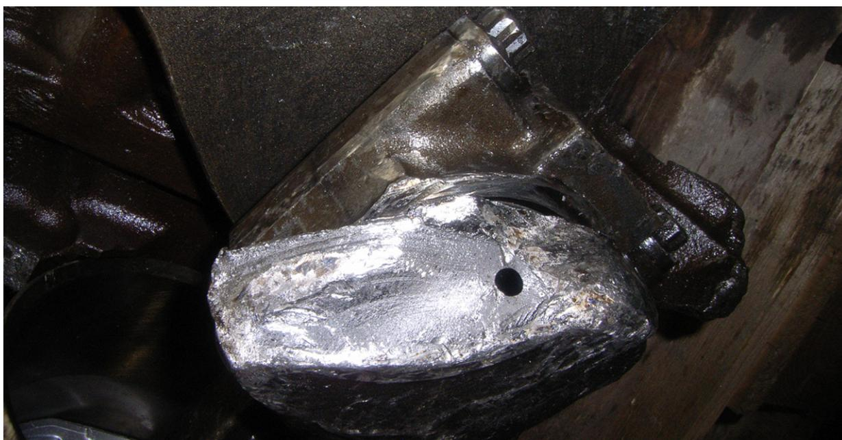
Figure 3: Crankshaft fracture face
