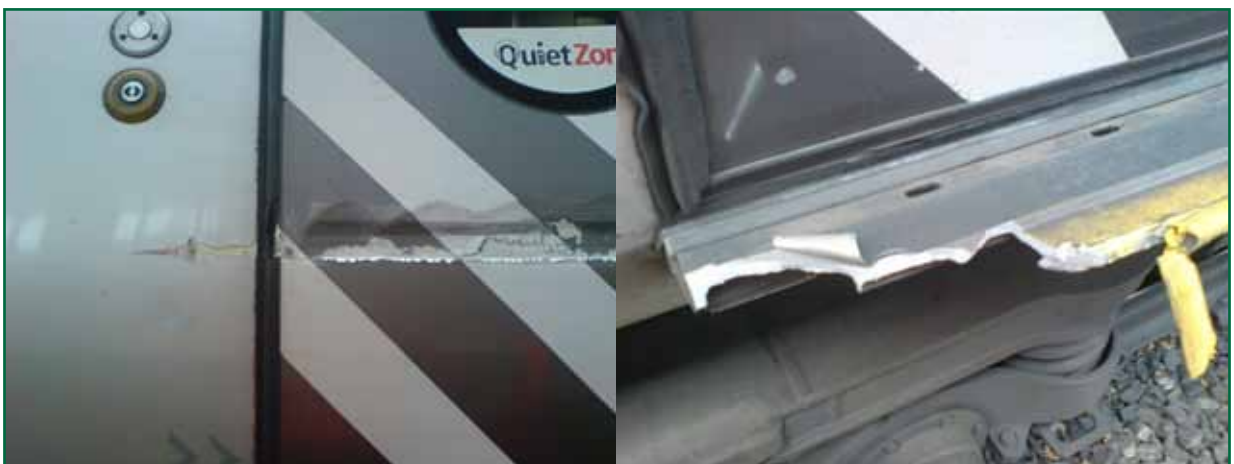
Figure 5: Damage to Super Voyager 221112 (image courtesy of Virgin Trains)
