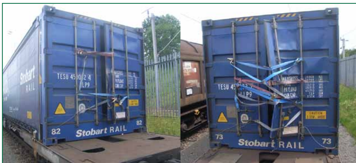
Figure 2: Damaged container doors
