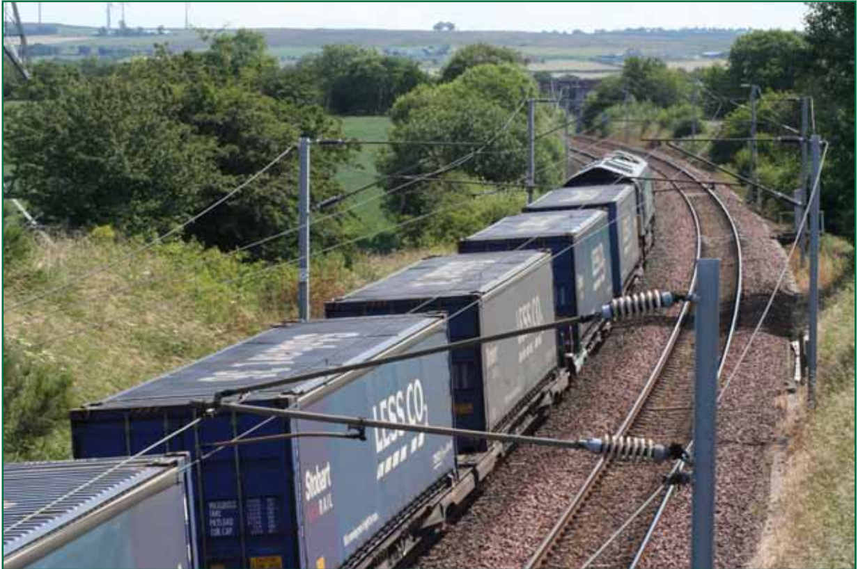
Figure 7: IKA wagons and 45 foot containers (image courtesy of Direct Rail Services)
