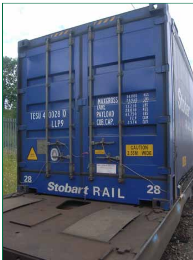
Figure 6: Door handle arrangements on a container
