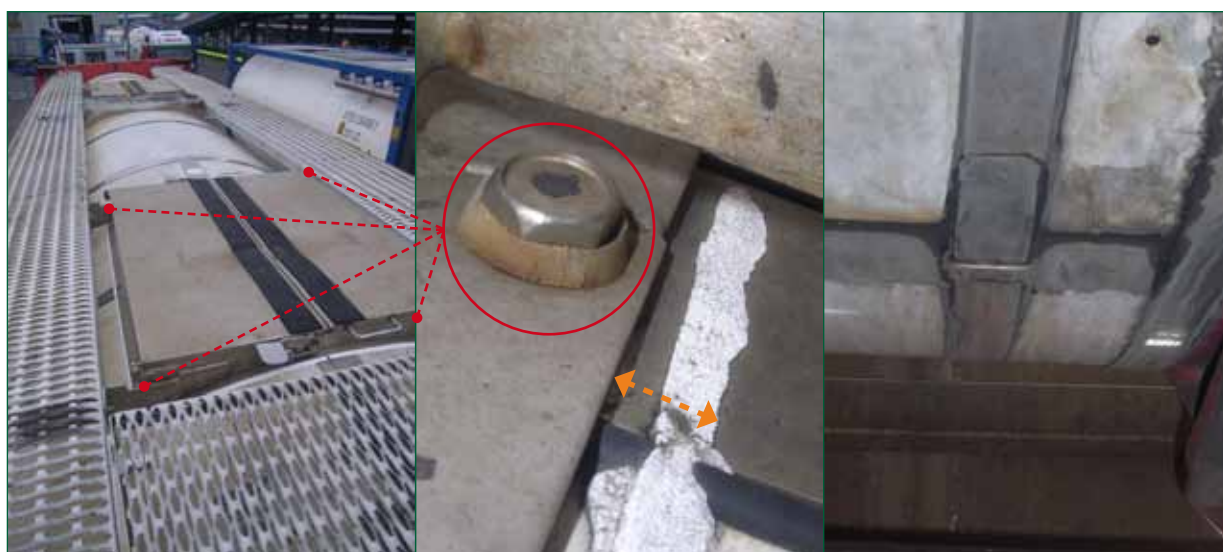
Figures left to right: 4a: top door of tank; 4b: securing screw for one side of the retaining straps; 4c: strap on underside of the tank secured by two rivets
