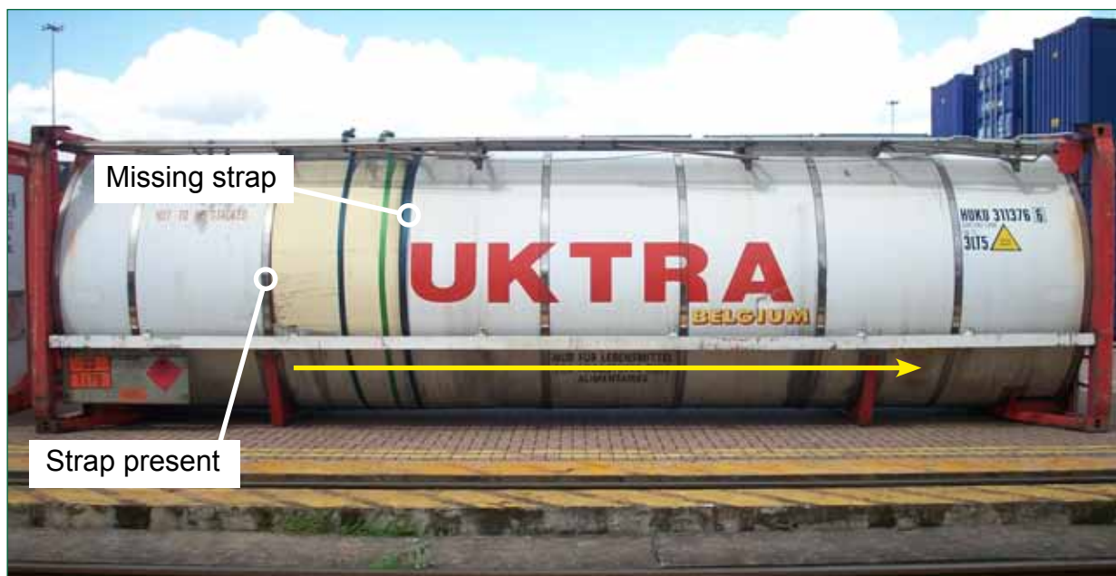
Figure 3: Image of the tank taken at Trafford Park, Manchester (direction of travel at the time of the incident at Carluke indicated with yellow line).
