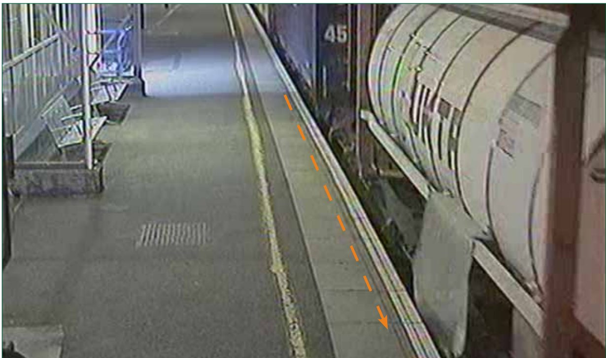
Figure 2: Image of the 'A' panel of the tank (located on the side opposite to that from which the panel was removed at Carstairs) passing through Manchester Piccadilly station platform after the train had been authorised to proceed without restriction. Direction of travel indicated by the orange arrow. By this time, the train had reversed direction at Crewe
