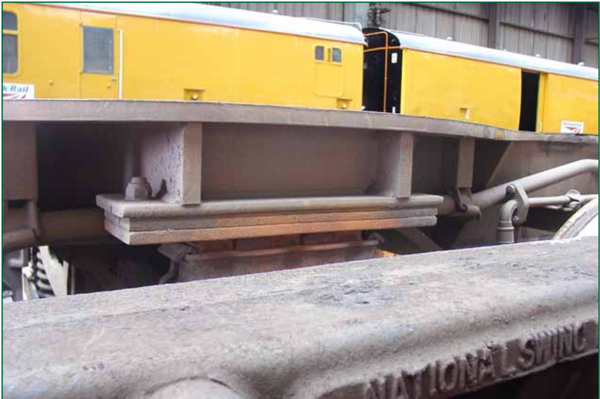
Figure 10: Sidebearer and packings fitted to leading left side of wagon 610117
