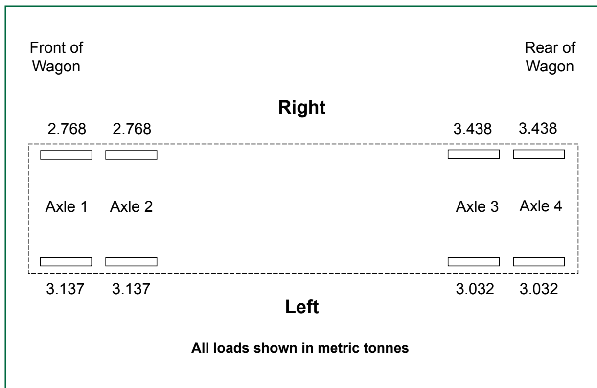
Figure 11: Wheel loads used in the dynamic analysis
