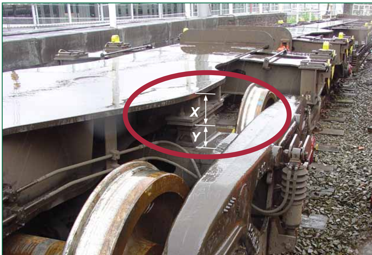
Figure 9: Right side of leading bogie of wagon 610117 showing (circled) sidebearer unit
