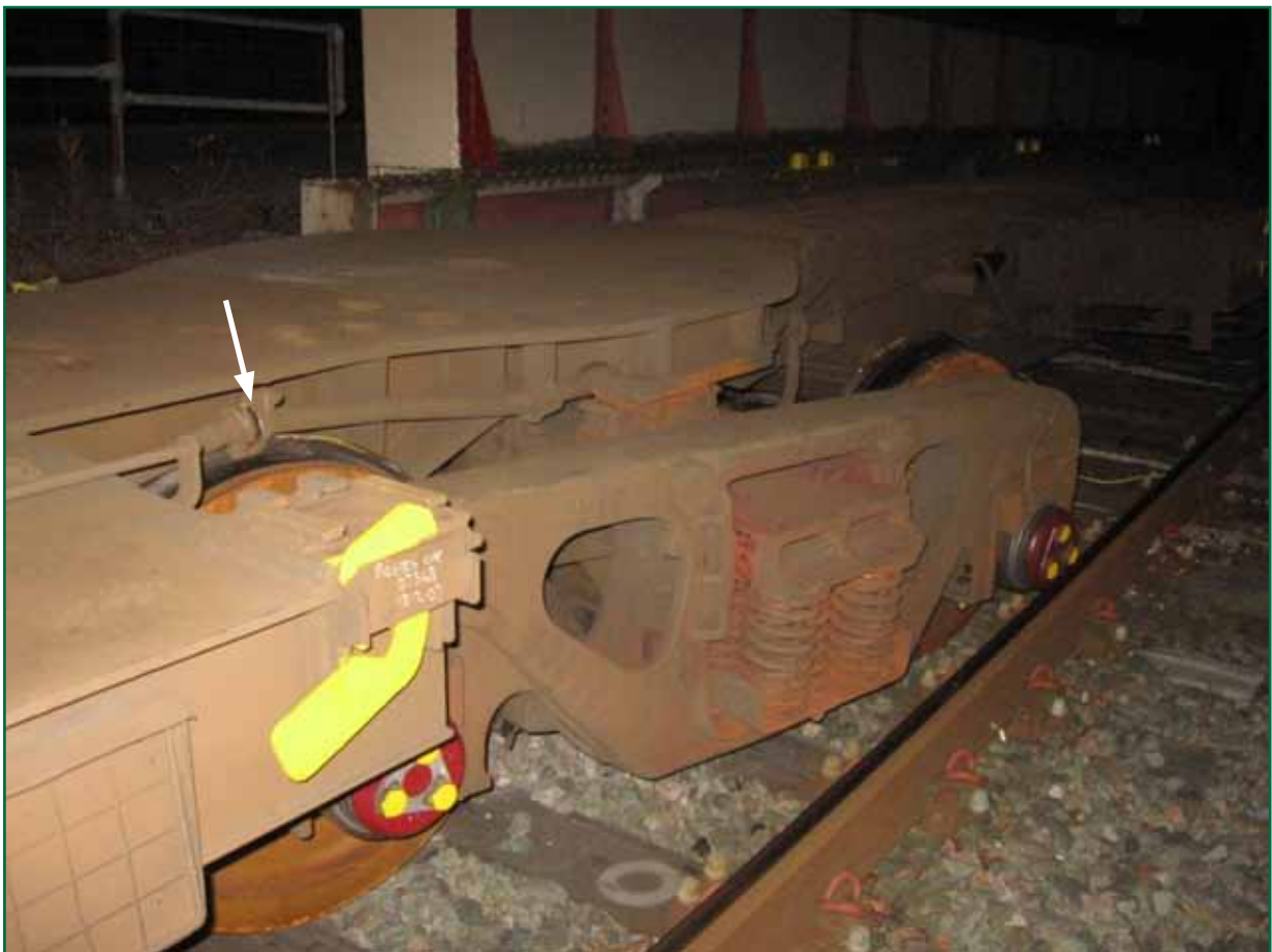
Figure 5: The derailed bogie with (arrowed) the fractured brake pipe (photograph courtesy of Network Rail)
