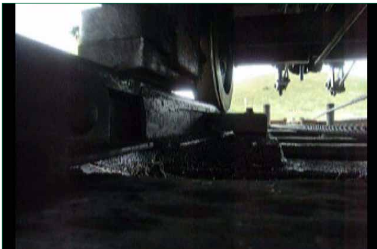
Figure 10: Flange contact between leading left-hand wheel and left-hand switch rail
