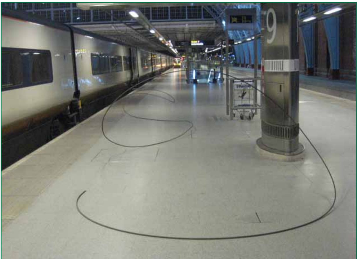
Figure 1: Photograph of displaced wire on platform (courtesy of Network Rail)
