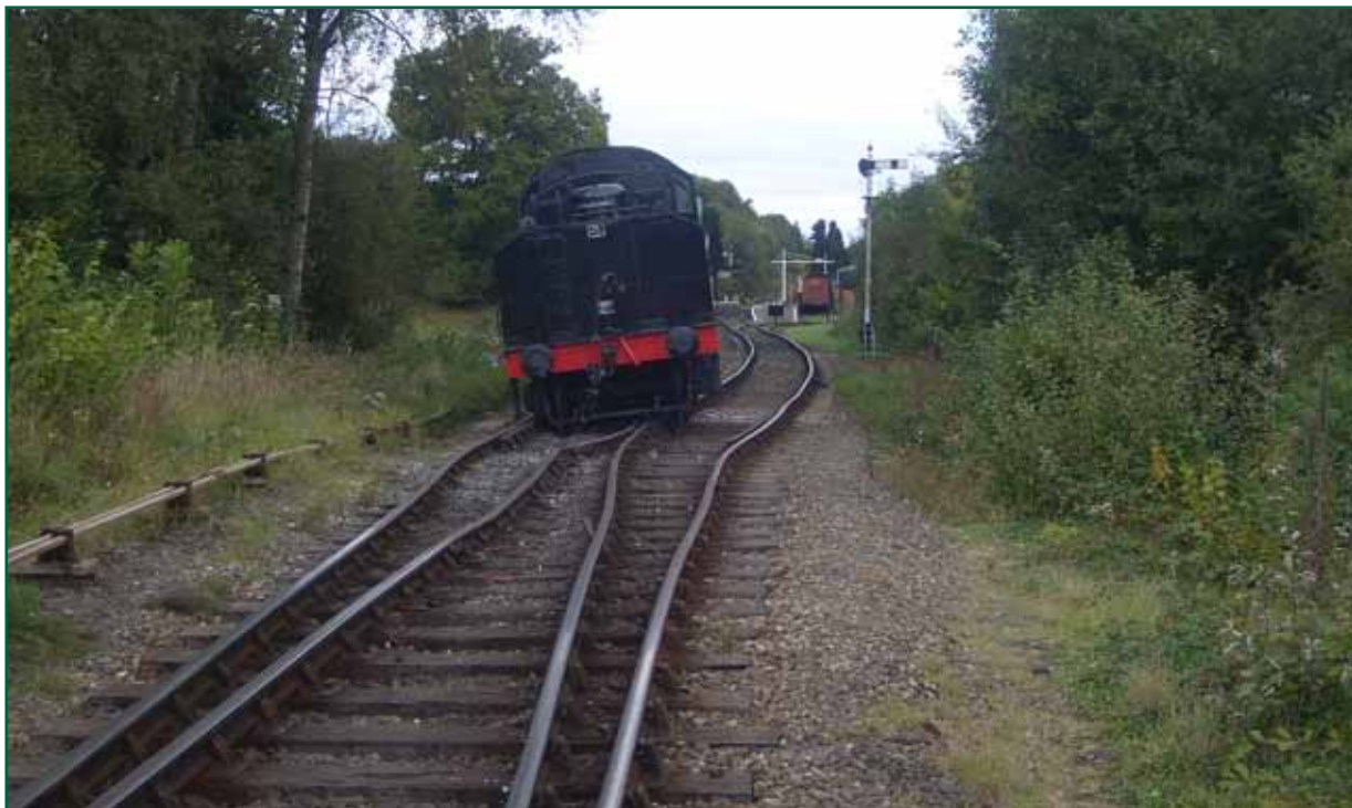
Figure 3: The derailed tender following removal of the train's coaches
