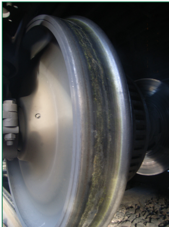
Figure 3: Contamination on one of the wheels of the main-line train
