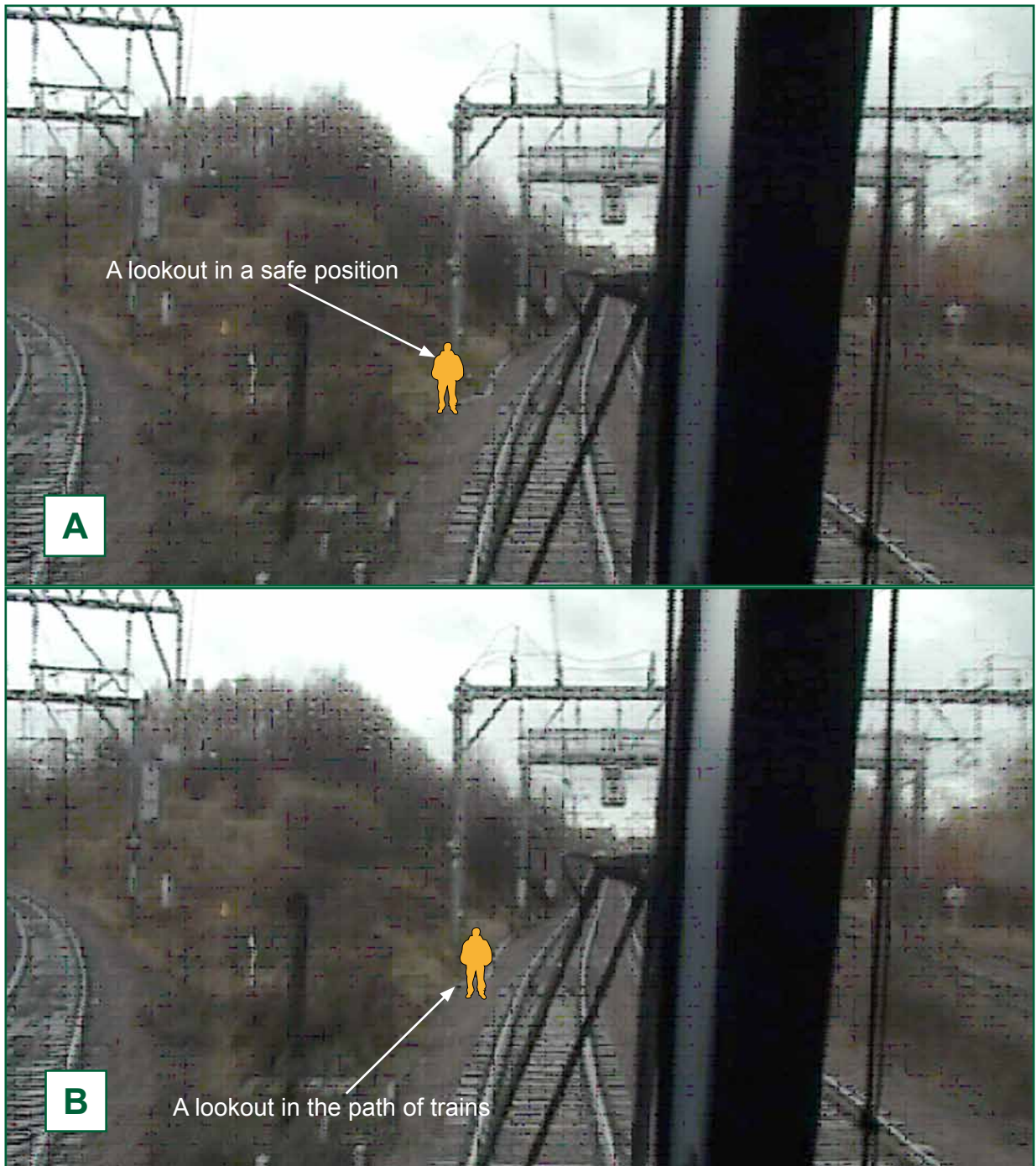
Figure 12: The view from the cab showing a lookout in a safe position (A) and in the path of trains (B)
