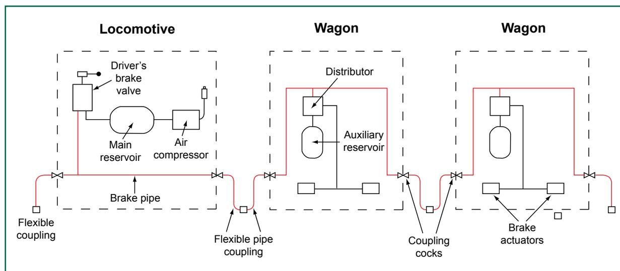
Figure 18: Simplified schematic diagram showing a single pipe system
