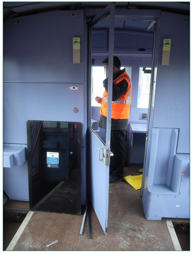
Figure 4: Glass window ejected from door following collision
