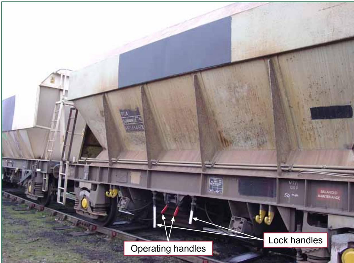
Figure 4: Wagon 14513, showing door control and locking handles
