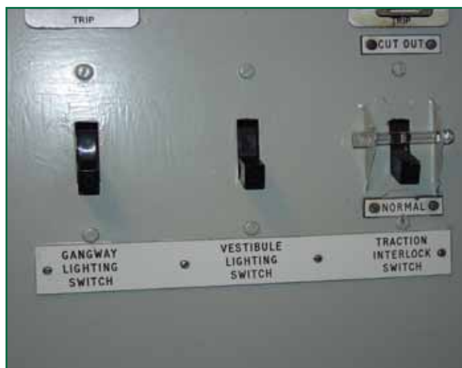
Figure 1: Switches on cab bulkhead of class 317, showing TIS in normal position with glass seal intact
