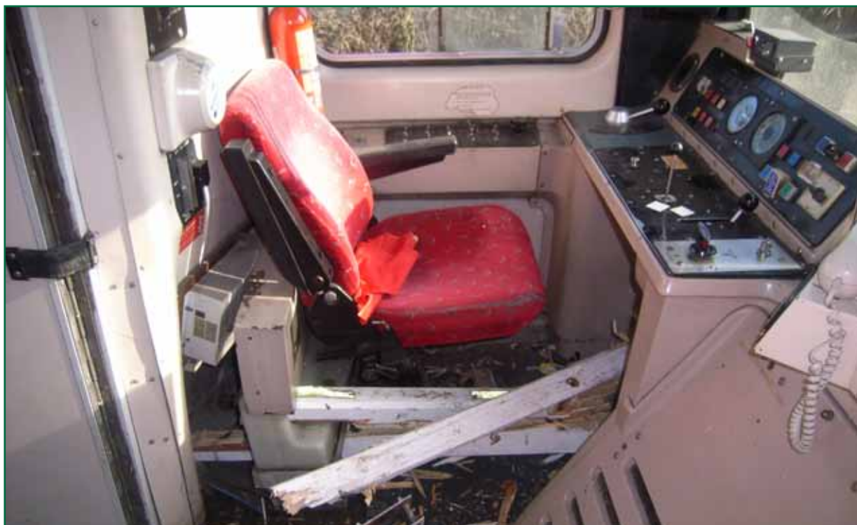
Figure 1: Cab interior following collision with level crossing gate
