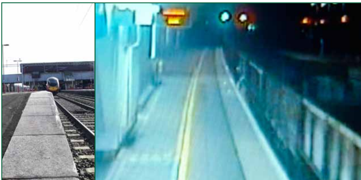
Figure 3 (left): initial impact mark and scrape marks on platform 4 at Birmingham International station. Figure 4 (right): wagon 112107 colliding with the up platform 4 at the same station. The wagon door had already fallen from the 90° to the 180° position.
