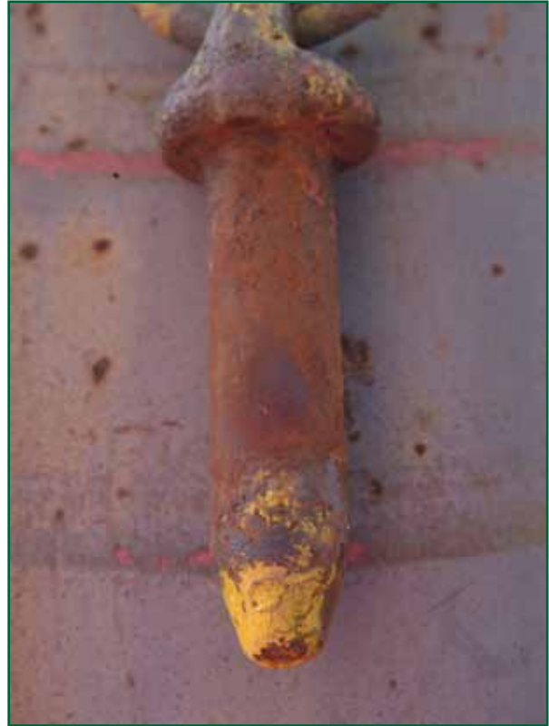
Figure 8: one of the three disengaged incident wagon pins found hanging at the side of the open wagon door
