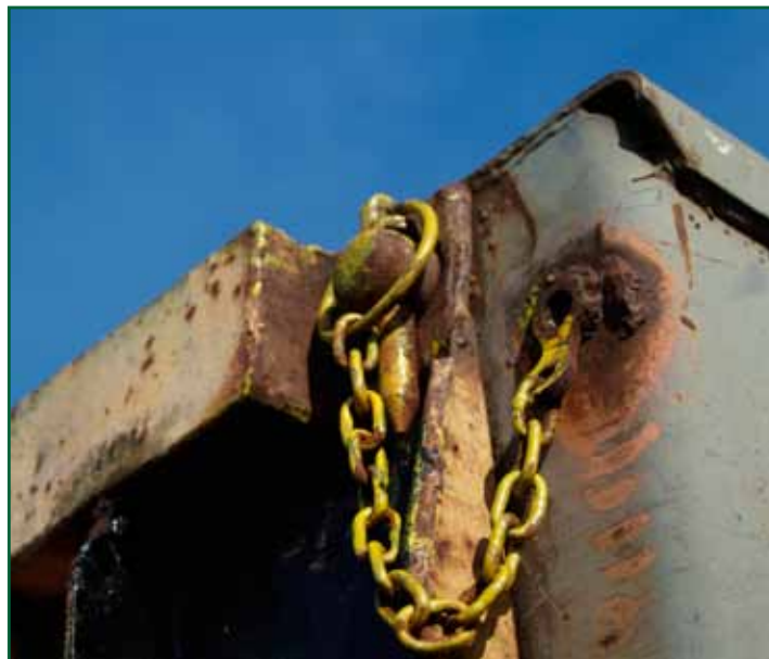
Figure 1: the pin passing through the spigot, shown in the fully engaged position and securing the door
