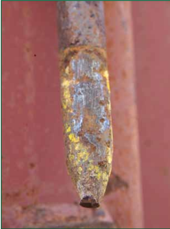
Figure 7: reference sample used to show contact marks after pin had been forcibly removed
