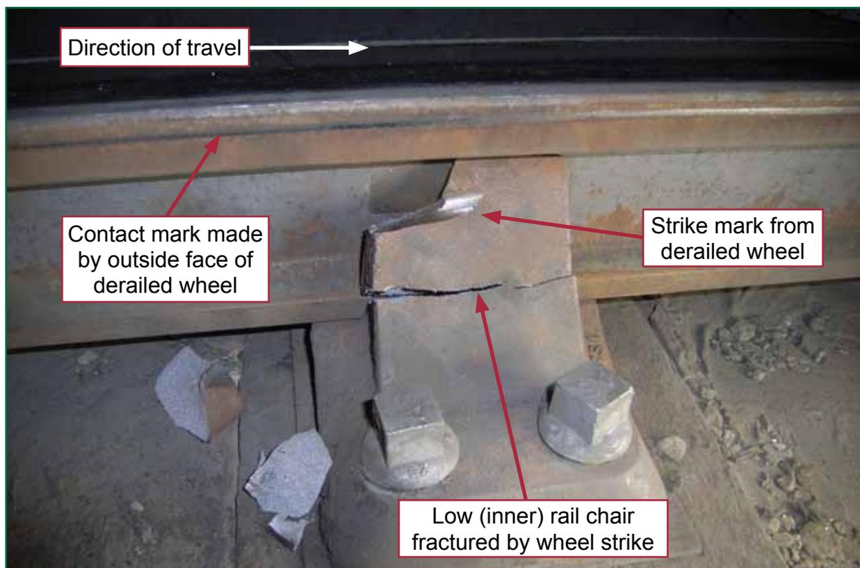
Figure 5: Left-hand wheel tread corner strike mark on low rail chair
