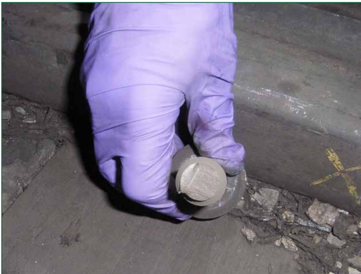
Figure 8: Fractured screws showing signs of fatigue failure
