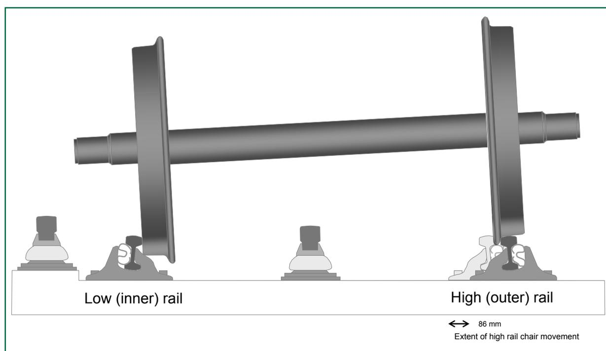
Figure 6: High (outer) rail movement, showing normal chair position and subsequent position of an unsecured chair allowing gauge to widen dynamically.
