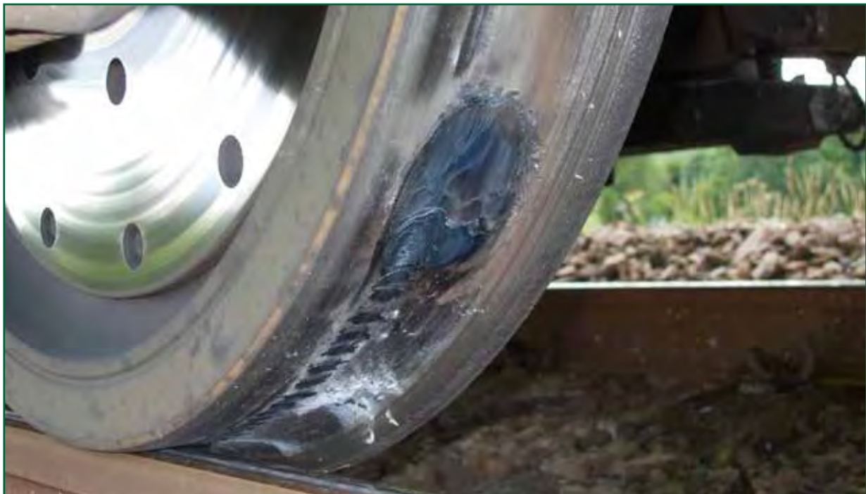
Figure 6: Damage to the wheel tread of HST power car 43041
