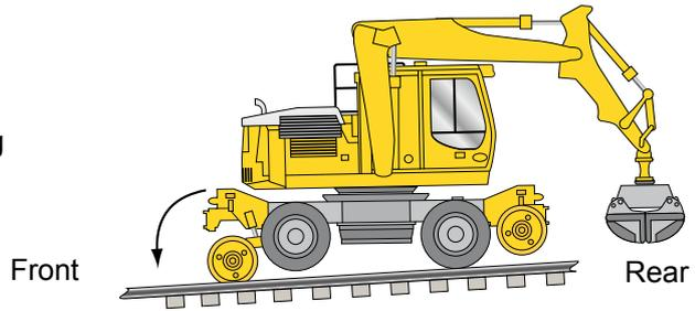
**Figure 14 f** - The machine operator raises the front rail wheels fully up and manoeuvres the RRV forward and backwards to re-align the rear rail wheels.
