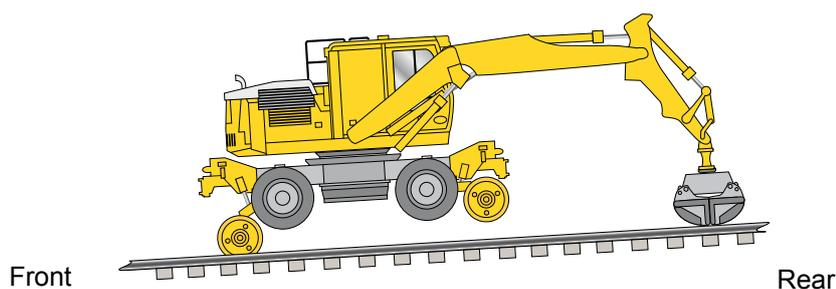
**Figure 14 o** - The machine operator lowers his boom arm and clam bucket onto the sleepers in the area between the running rails of the down line (at the rear end of the RRV). This lifts the RRV up and the rear rail wheels are then placed onto the track.
