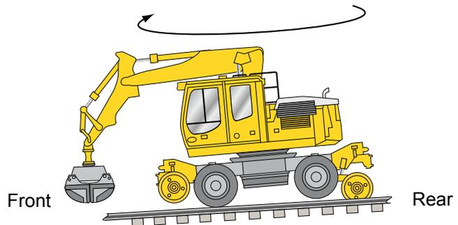
**Figure 14 h - i** - The machine operator swings the cab to the front of the RRV
