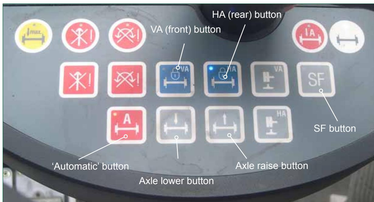
Fig 13: Rail (ZW) control panel indicating axle operation buttons
