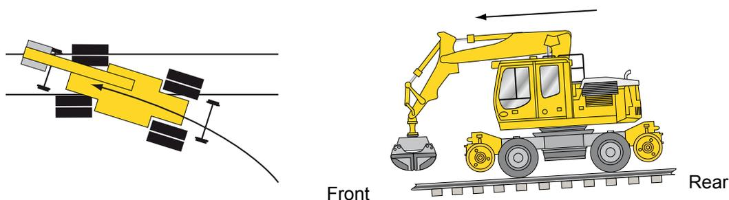
**Figure 14 a/b** - Rail mode is selected on the ZW box. The RRV is driven onto the RRAP front end first. The machine controller is not present. The RRAP is on a 1 in 50 max gradient
