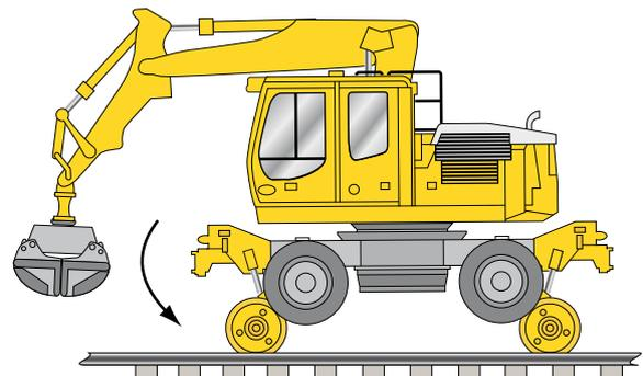
*Figure 9a - h: High-ride RRV - correct method of on/off-tracking*
