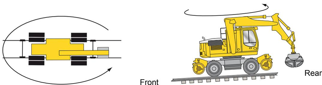
**Figure 14 c/d** - The cab is swung to the rear of the RRV. The machine operator believes that the rear rail wheels are in line with the track: they are not.
