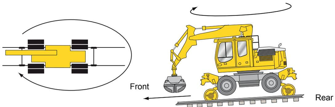
**Figure 14 r - s** - The machine operator quickly swings the cab to the front of the RRV (in the direction of travel).
