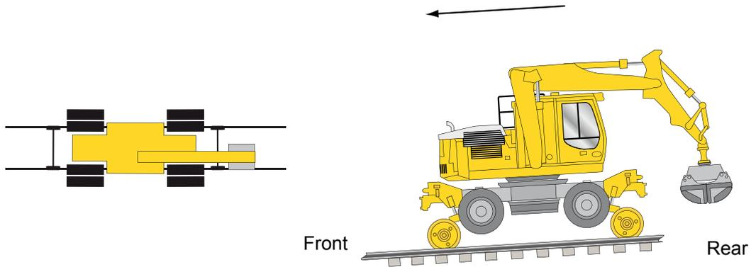
**Figure 14 p - q** - The RRV begins to run away as it is in a free-wheeled state and on the track.
