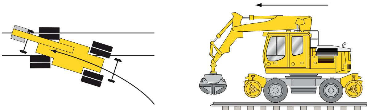
**Figure 9 a & b** - Rail mode is selected on the ZW box. The RRV is then driven onto the RRAP, front end first. The machine controller should be present.
