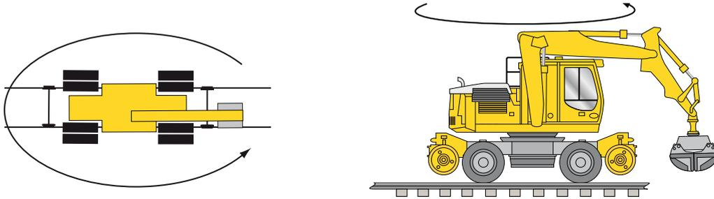
**Figure 9 c & d** - The cab is swung to the rear of the RRV and the rear rail wheels are lined up with the track using the road wheels to manoeuvre the machine.
