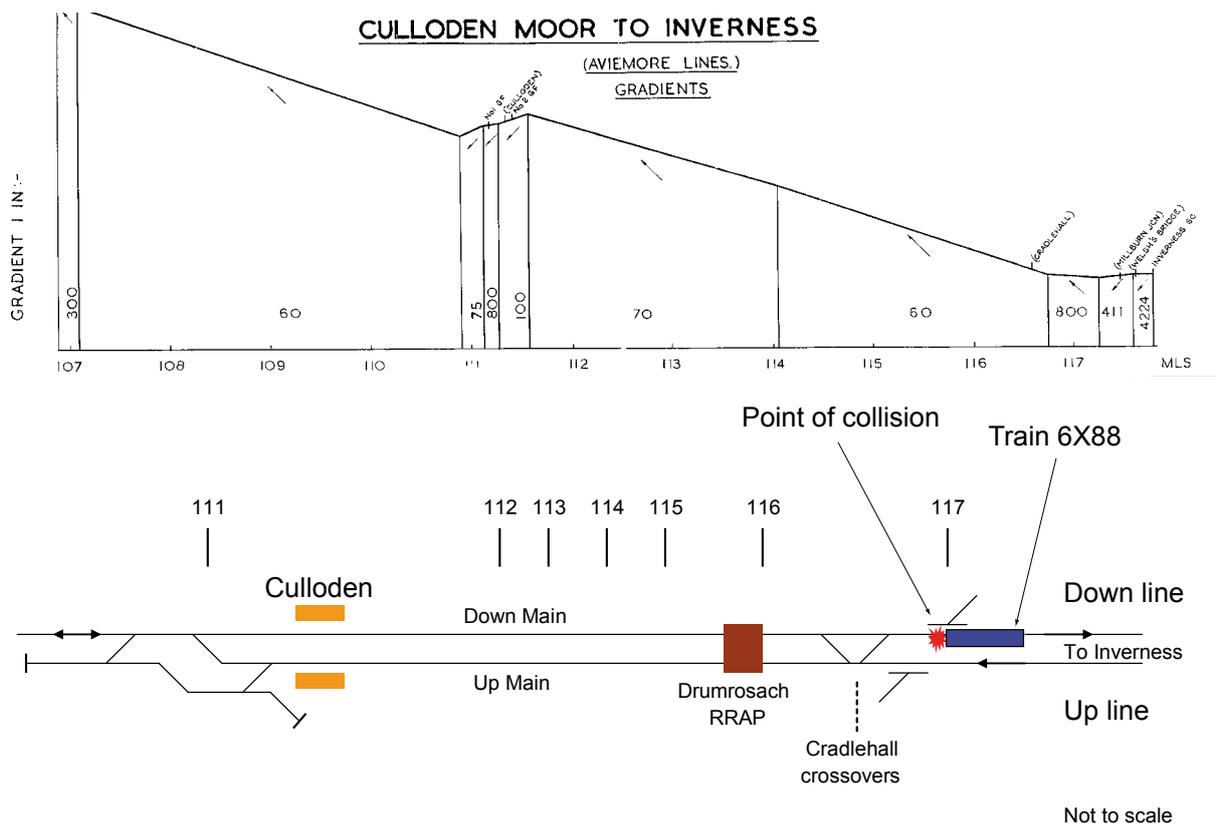
Figure 3: Track plan between Inverness and Culloden showing the RRAP and the accident site with associated gradient information
