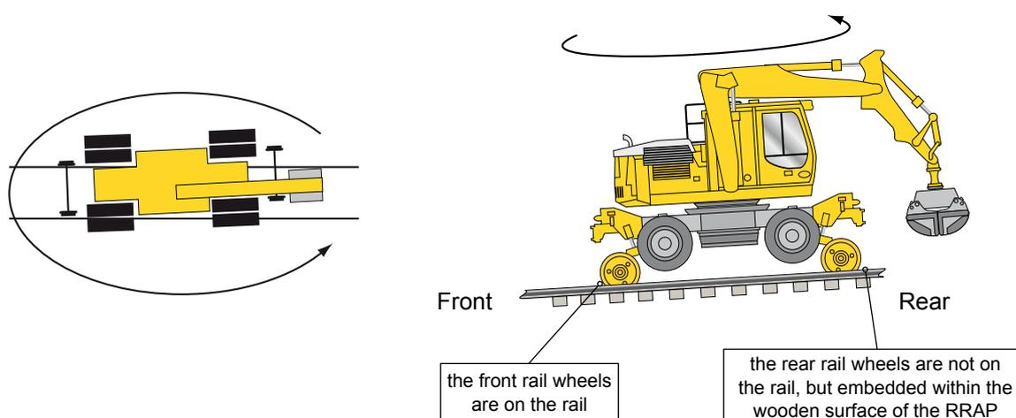
**Figure 14 m - n** - The machine controller arrives at the RRAP and tells the machine operator that the RRV rear axle wheels are not on the track, but in the wooden surface. The machine operator swings the cab to the rear of the RRV.
