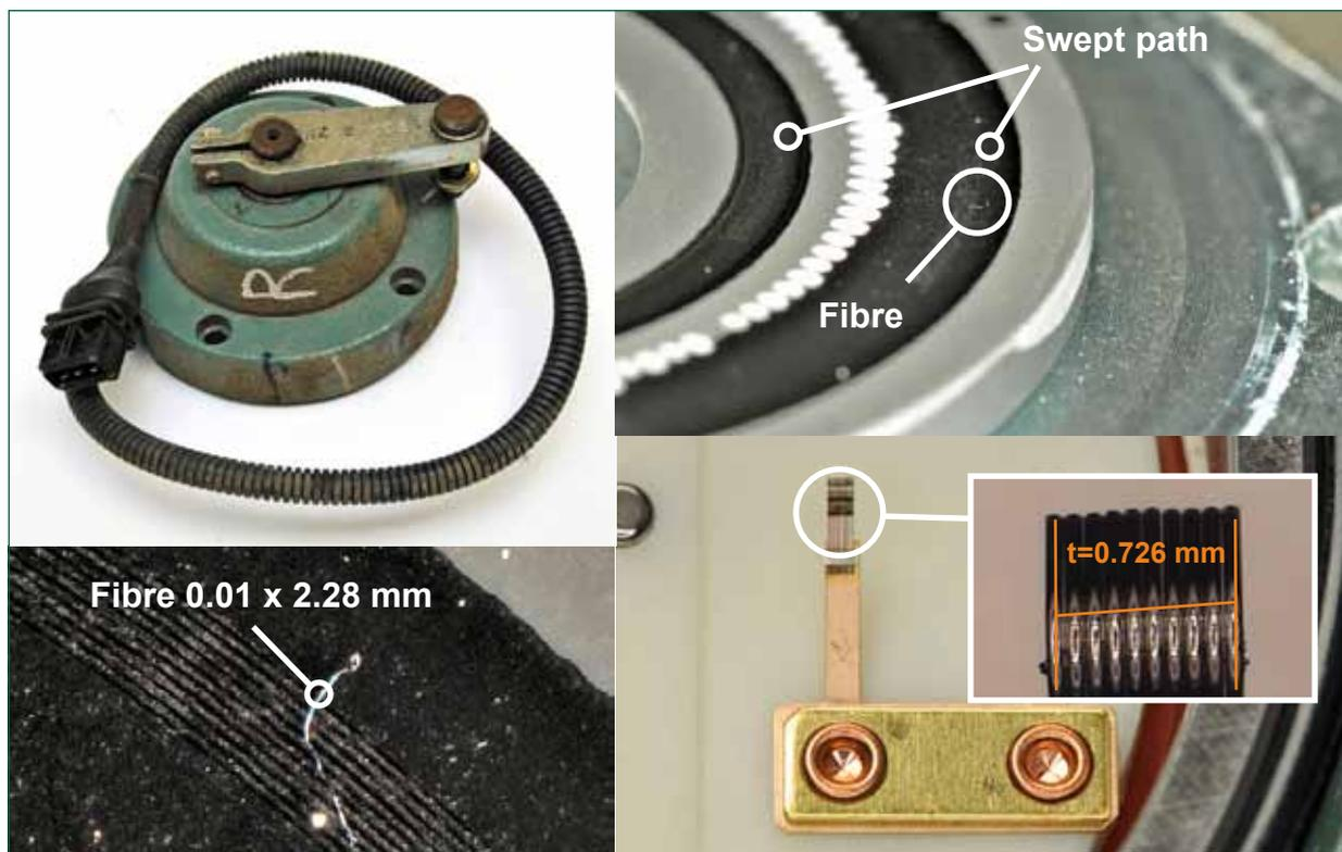
Figure 10: Photographs (clockwise from top left) of the 'third' potentiometer, swept path, wiper arrangement and track and fibre (with dimensions in millimetres)
