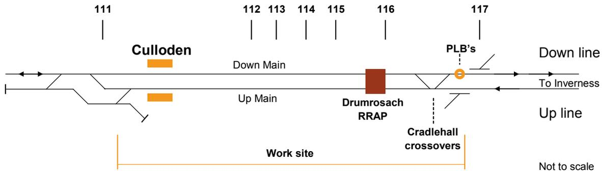
Figure 6: Track plan showing the possession and worksite limits for 20 July 2010
