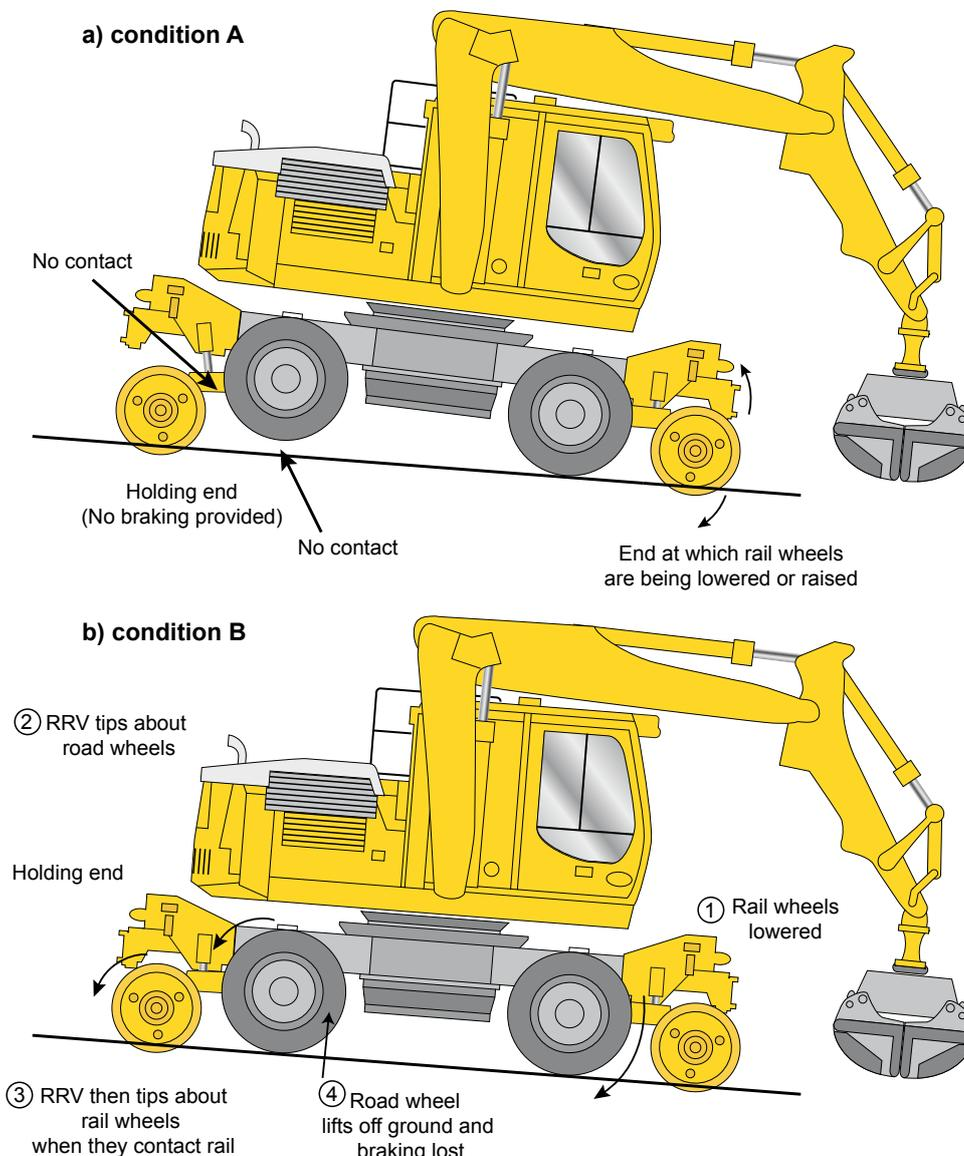
Figures 8a and 8b: High-rise RRV - on/off-tracking runaway conditions
