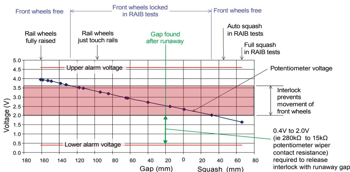
Figure 11: Graph showing relationship between voltage and road/rail wheel air gap
