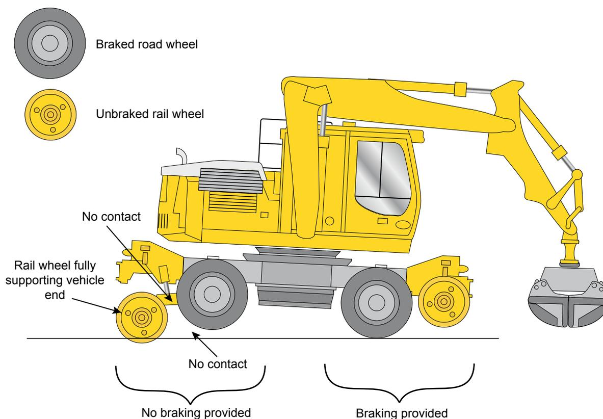
Figure 7: High-ride RRV - transition condition that results in no braking being provided at one end of the machine during on/off-tracking
