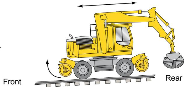
**Figure 14 g** - The machine operator believes that the rear rail wheels are now in line with the track. They are still not. The machine operator lowers the rear rail wheels onto the RRAP surface causing damage (figure 12). A gap of about 20 mm (inset) (paragraph 106) is left by the machine operator between the rear road and rail wheels (in accordance with the normal process during on-tracking).
