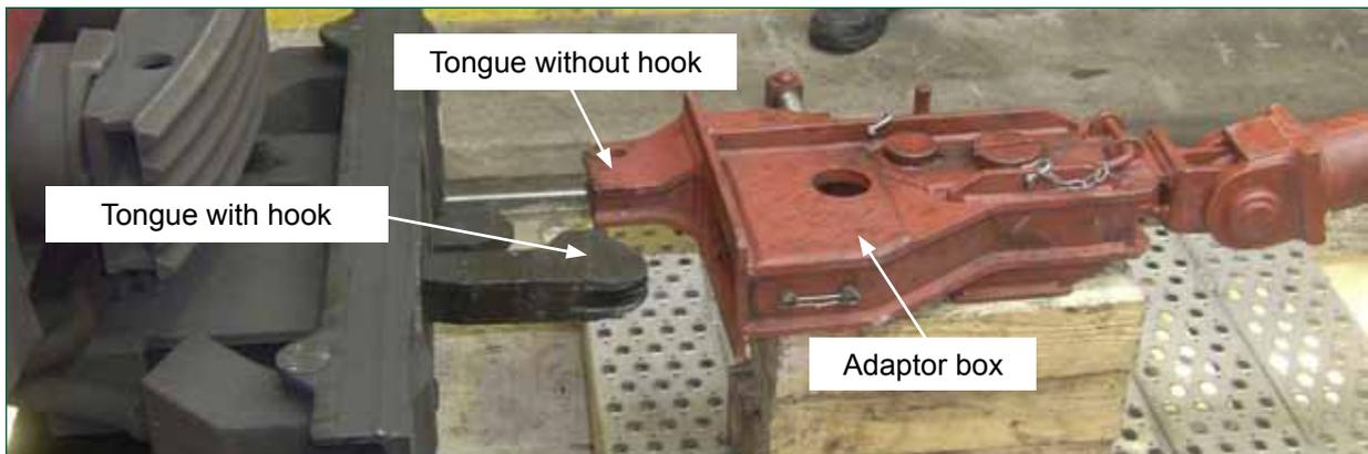
**a) Passenger train and adaptor box - Hooked tongue permits mechanical connection**
