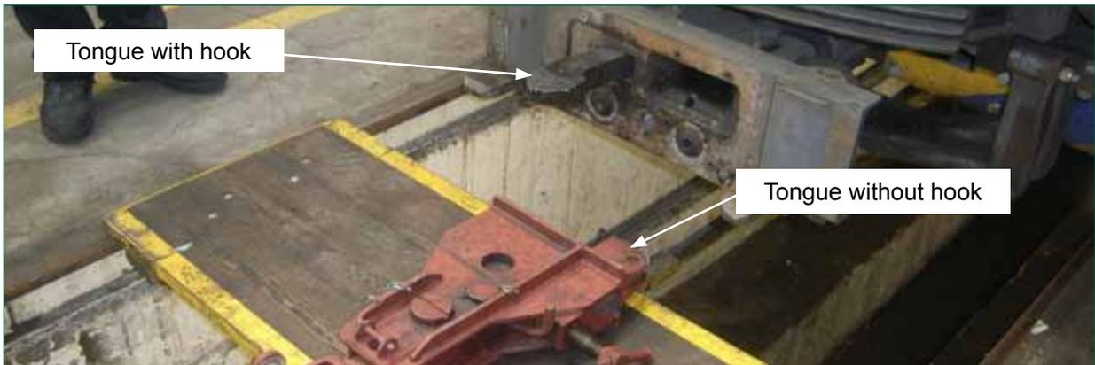
**b) Schoma locomotive and adaptor box - Hooked tongue permits mechanical connection**
