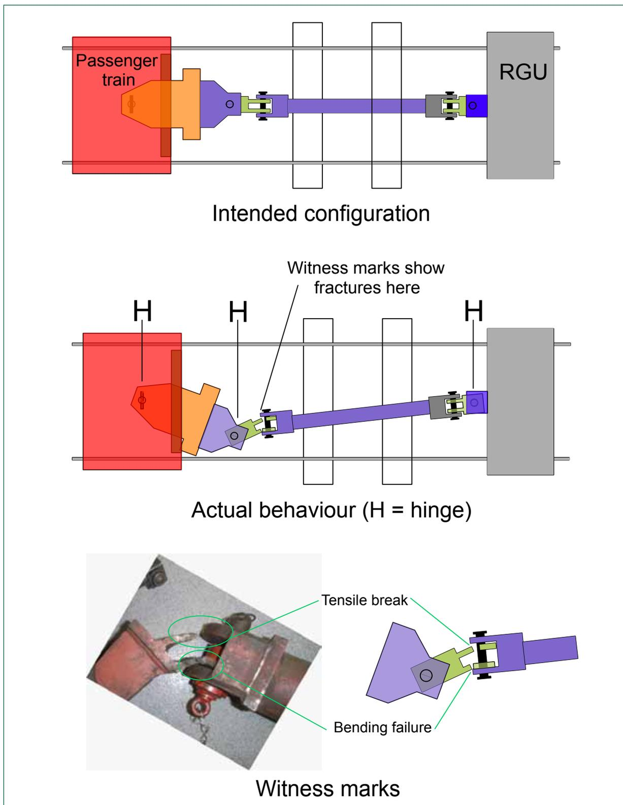
Figure 15: Lateral coupling deflection (phase 2 of breakage).
