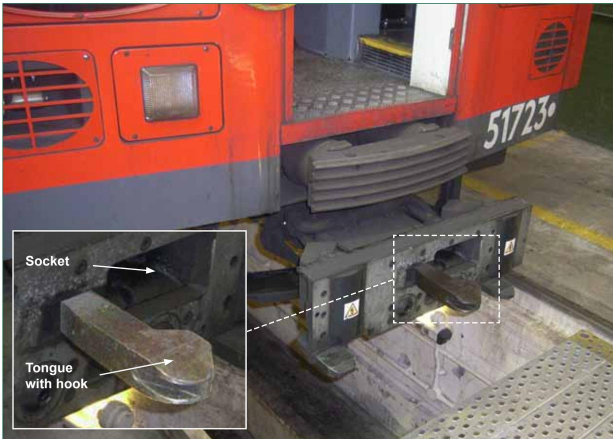
Figure 10: Wedgelock coupler.
