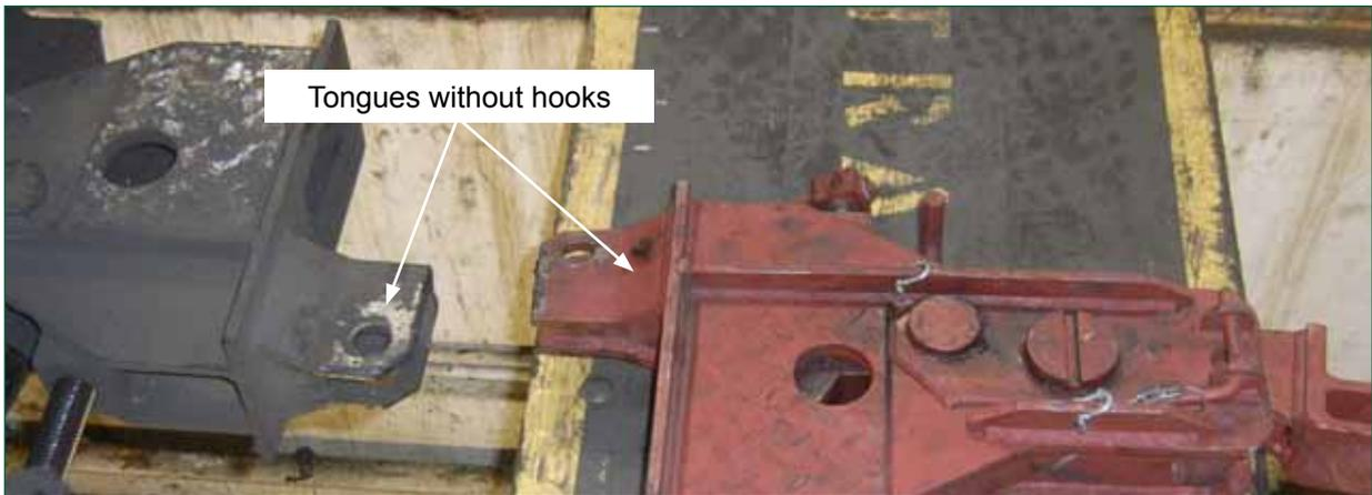
**c) Battery locomotive and adaptor box - Mechanical connection impossible because neither tongue has a hook**
