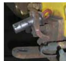
Deformed upper clevis plate allowed tow bar to fall onto track
