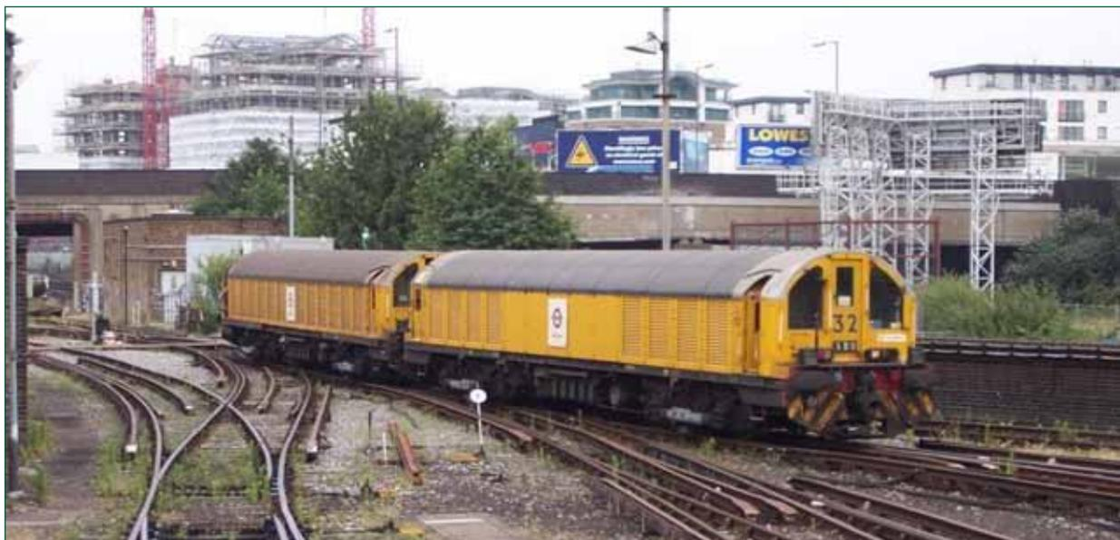
Figure 5: Two battery locomotives (image courtesy of Tube Lines).
