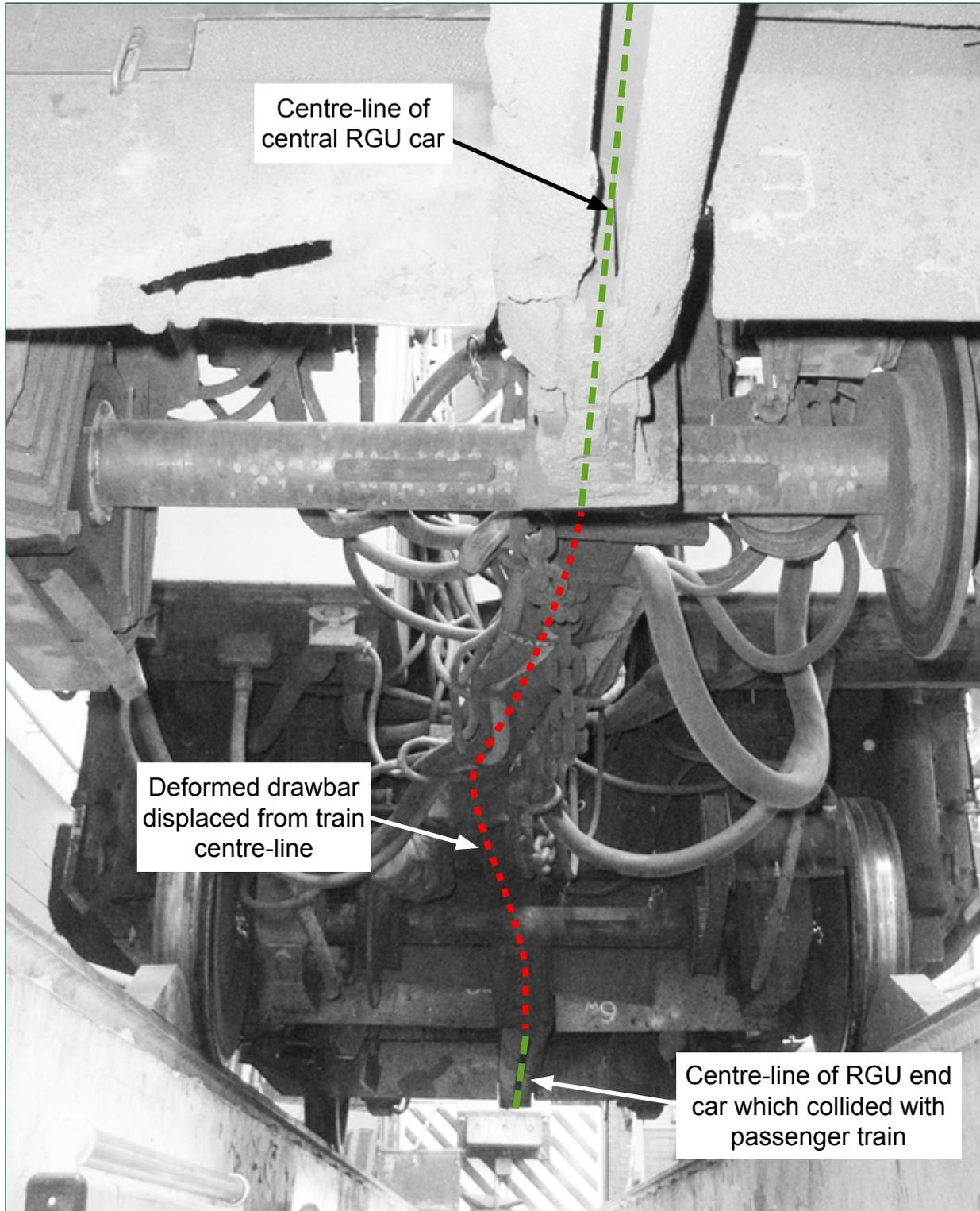
Figure 18: Deformed drawbar on RGU.
