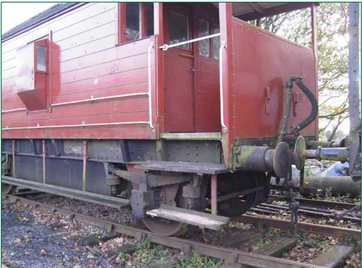
Figure 2: The brake van involved (note: the footstep was sanded after the accident)
