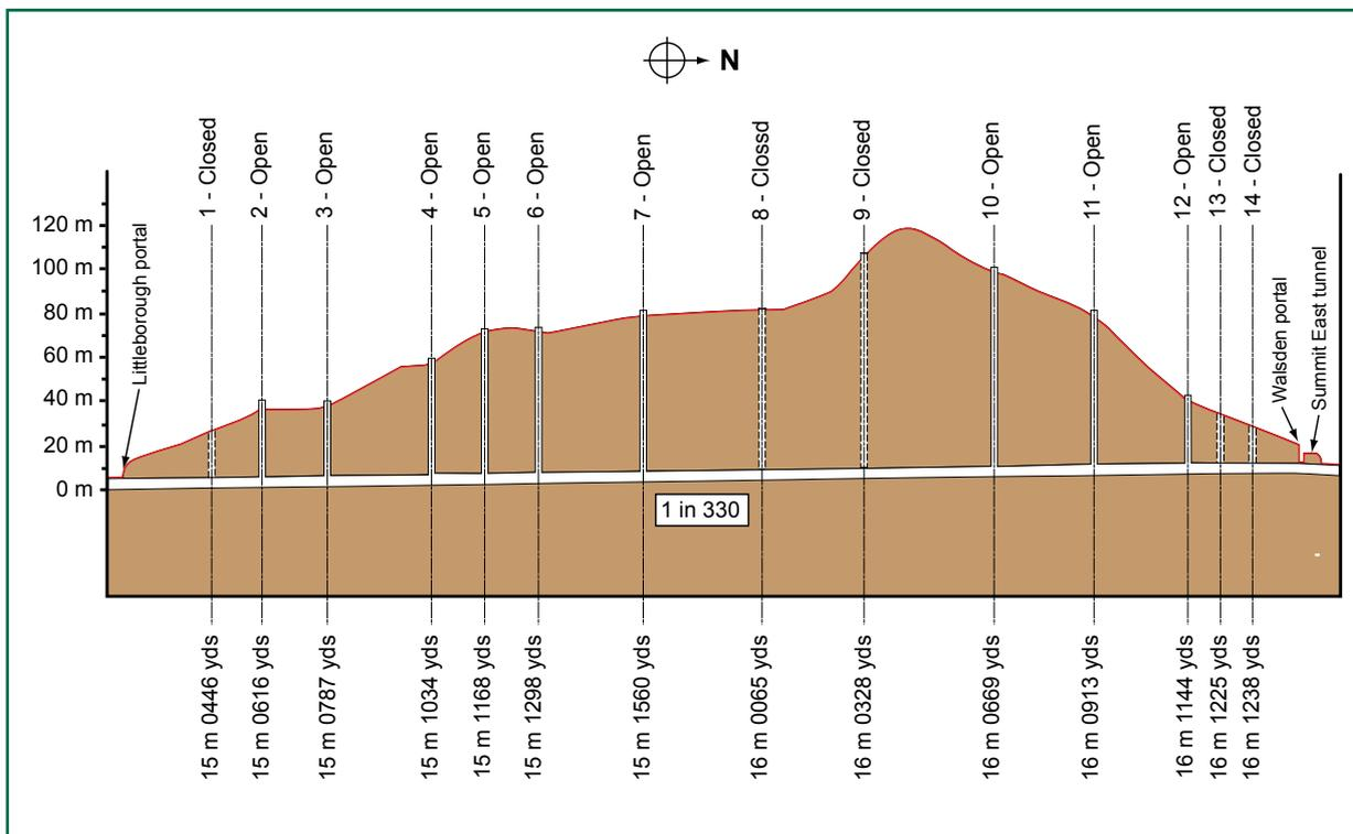
Figure 4: Profile of Summit tunnel showing the location, depth and type of each shaft
