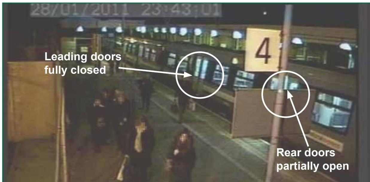
Figure 7: CCTV still showing accident door at the rear of the train partially open (and partially obscured by a station information sign) and leading door closed.
