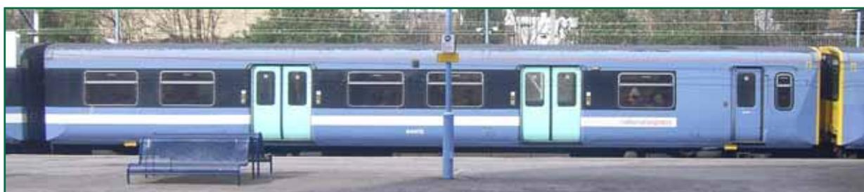
Figure 6: Class 315 EMU with doors at 1/3 and 2/3 positions.
