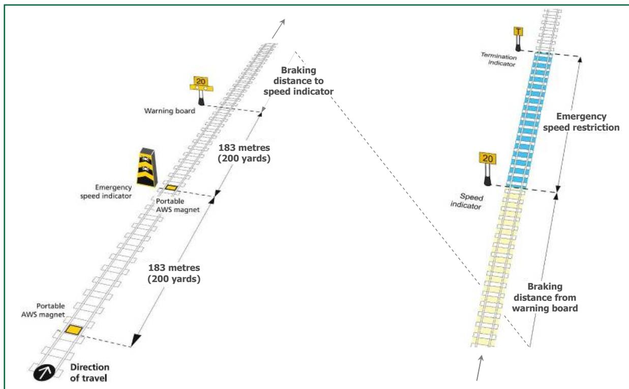
Figure 5a: Layout of the equipment required for an ESR (courtesy of RSSB)
