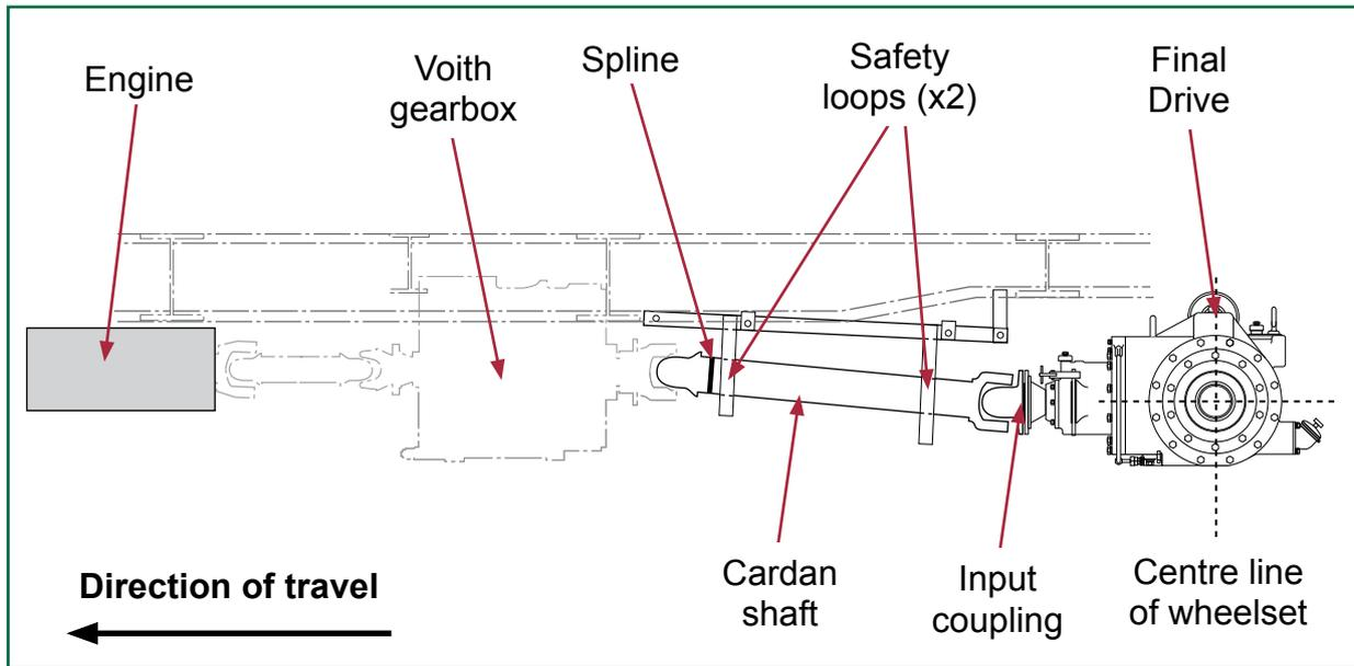
Figure 3: Drive arrangement on Class 14x
