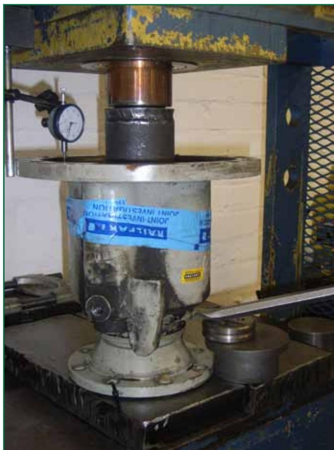
Figure 11: End float measuring technique
