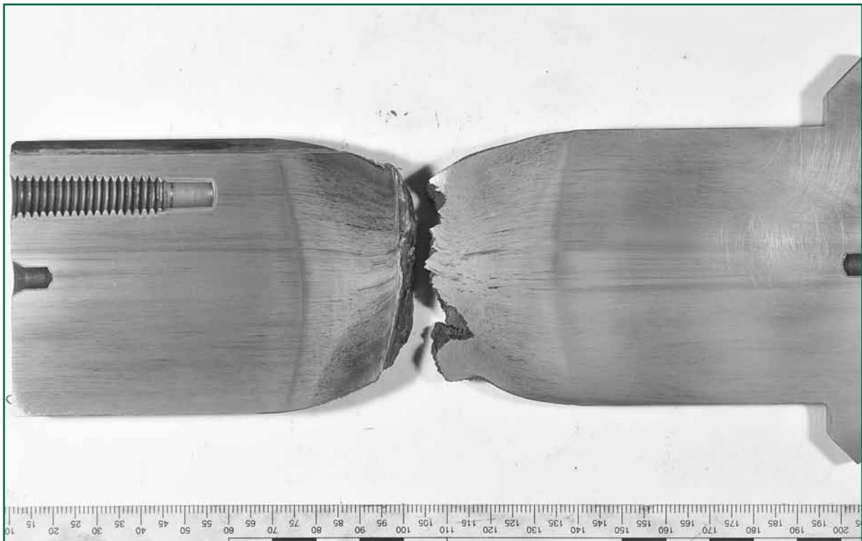
Figure 8: Section through the input shaft
