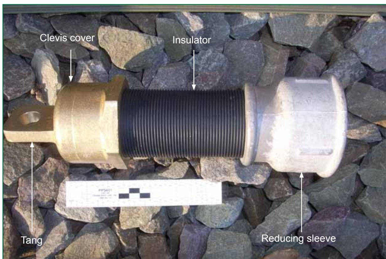
Figure 6: Bracket foot assembly
