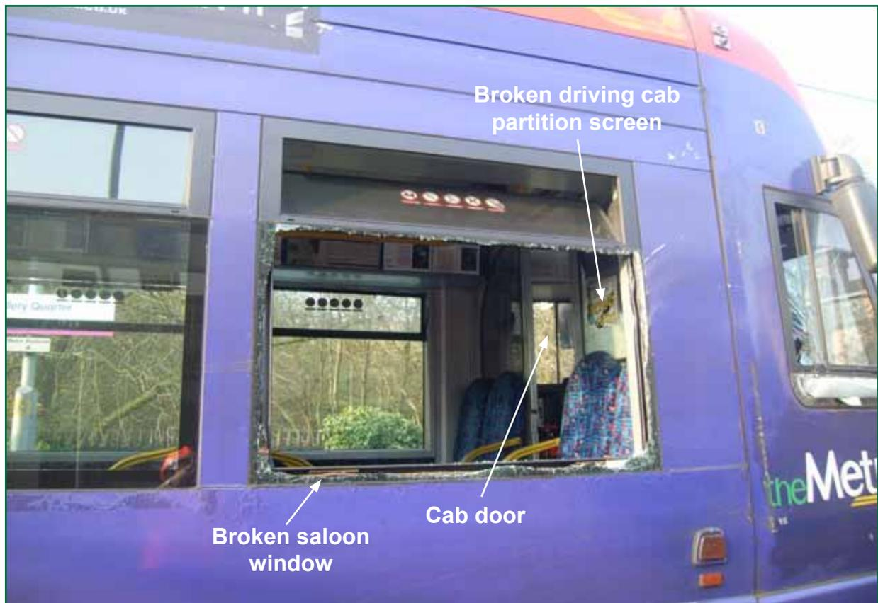
Figure 13: Damage to saloon window and driver's screen glass on the right-hand side leading end of Tram 13
