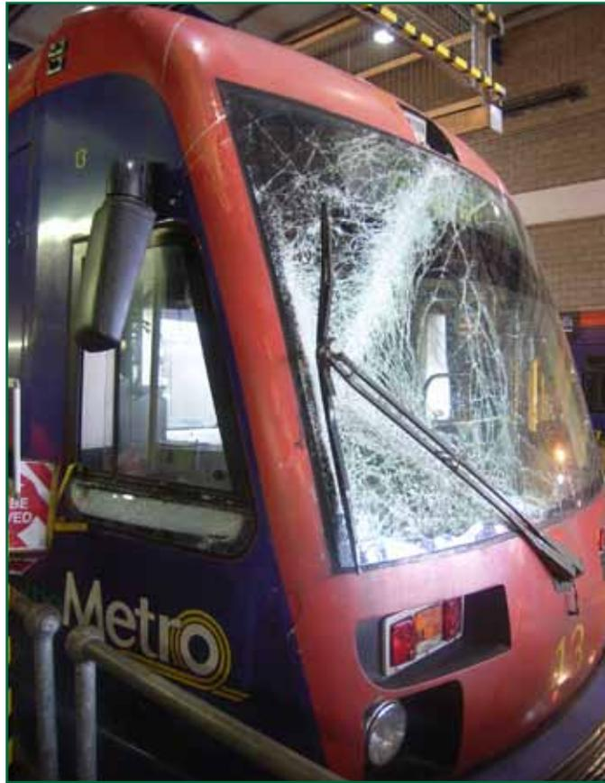
Figure 12: Damage to front windscreen and cab side window of Tram 13
