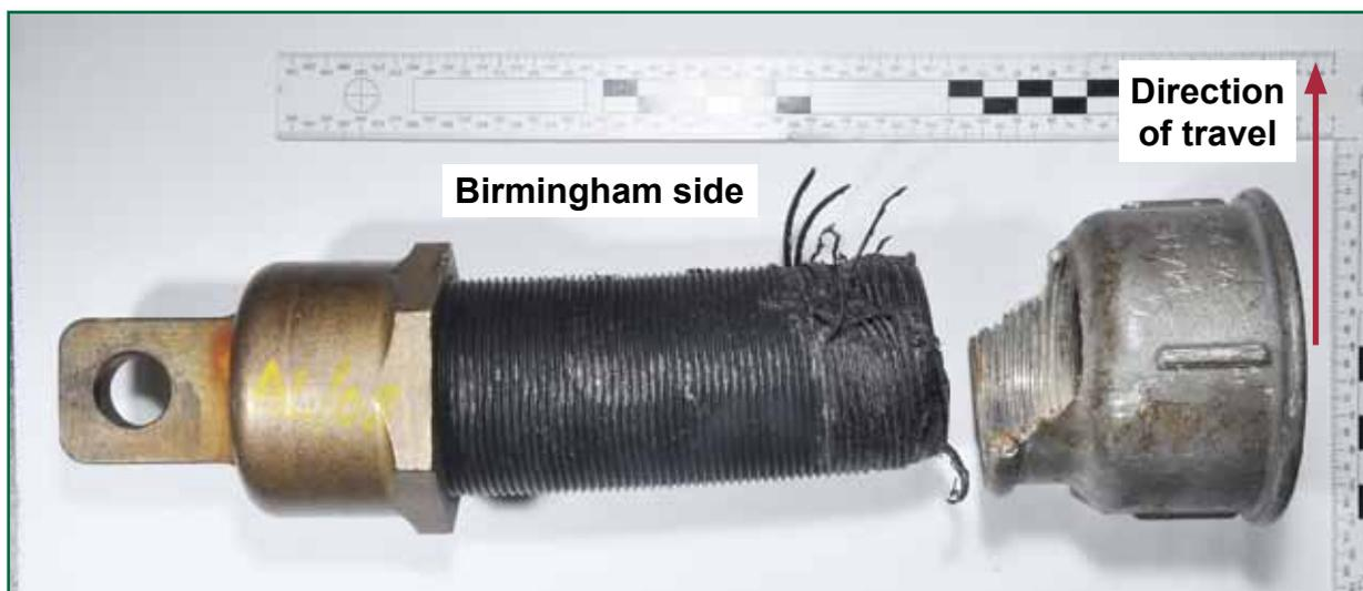
Figure 14: Damage to the bracket foot assembly of 18512 pole
