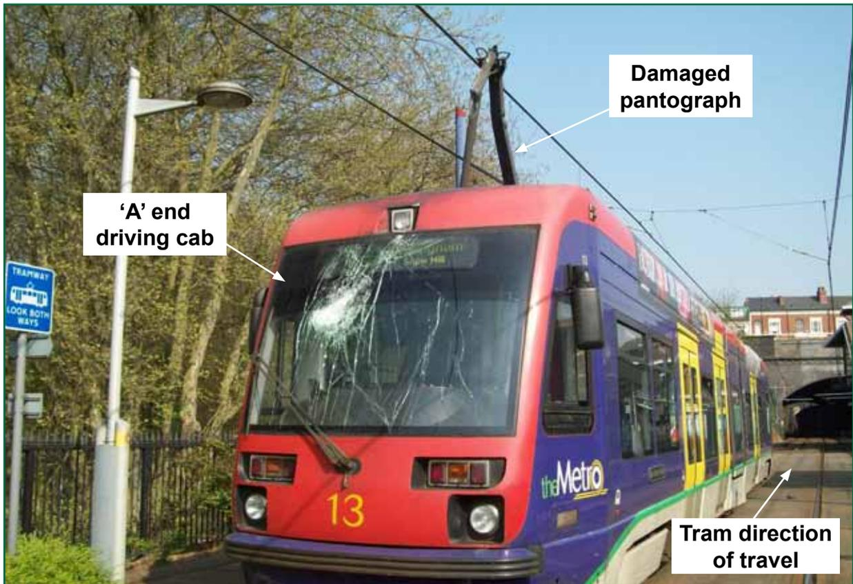
Figure 3: Damage to the trailing end of tram 13 (image courtesy of National Express Midland Metro)
