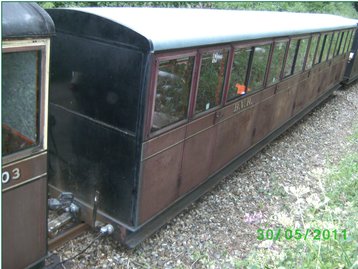
Figure 2: Derailed second coach (courtesy of the Bure Valley Railway)
