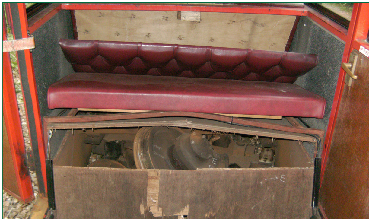
Figure 6: Incursion of the derailed bogie into the passenger accommodation (courtesy of the Bure Valley Railway)
