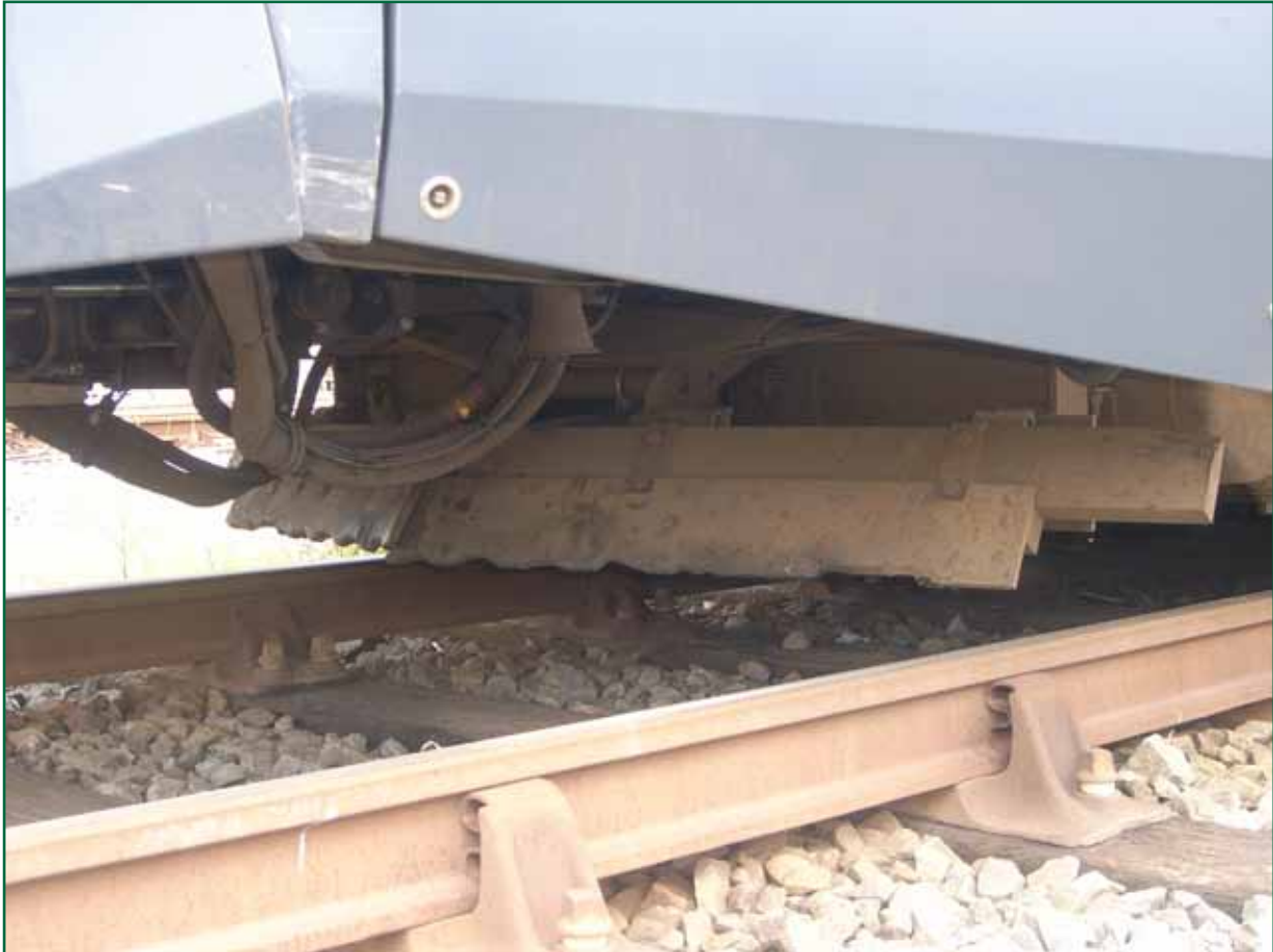
Figure 4: The under-run protector on the 'A'-end of tram 1002 (not at accident site); the notches in the rubber edge are caused by occasional contact with rail heads
