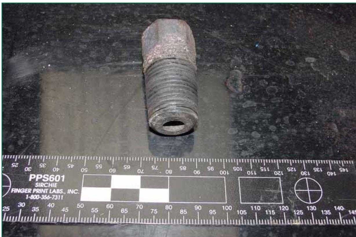
Figure 6: Fusible plug removed from 'Hawk'
