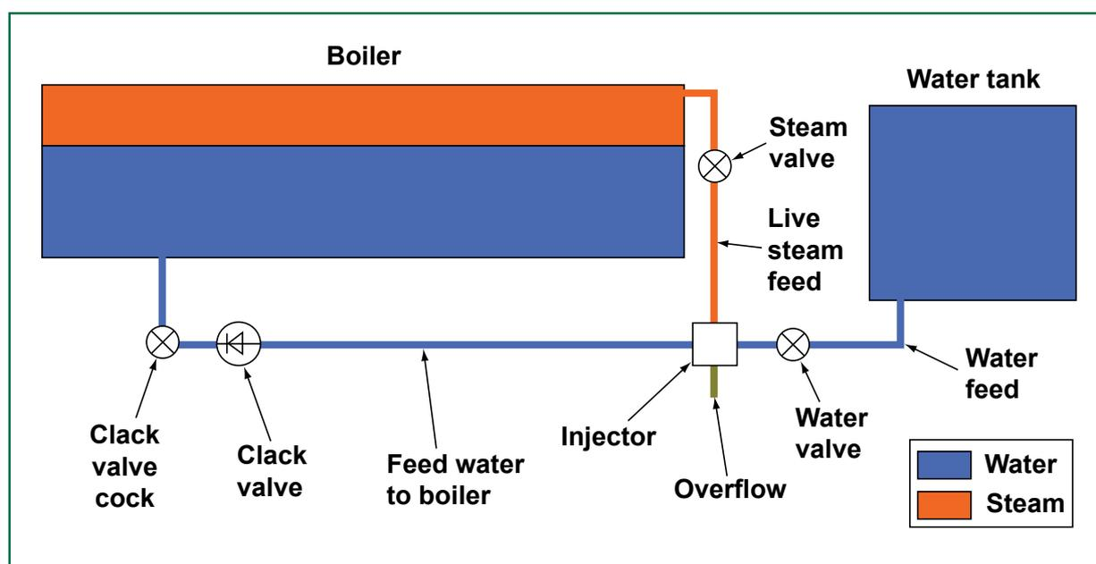
Figure 3: Schematic diagram of the water feed arrangements
