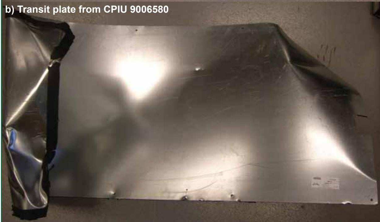
Figure 11: The transit plates that detached from containers CPIU 9006580 and 9006609 on train 4L68
