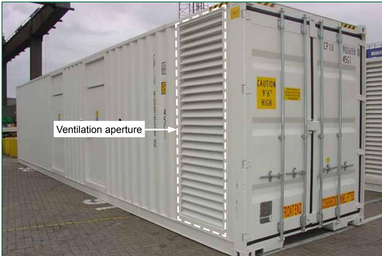
Figure 4: Container CPU 9006580 showing the location of the side ventilation aperture
