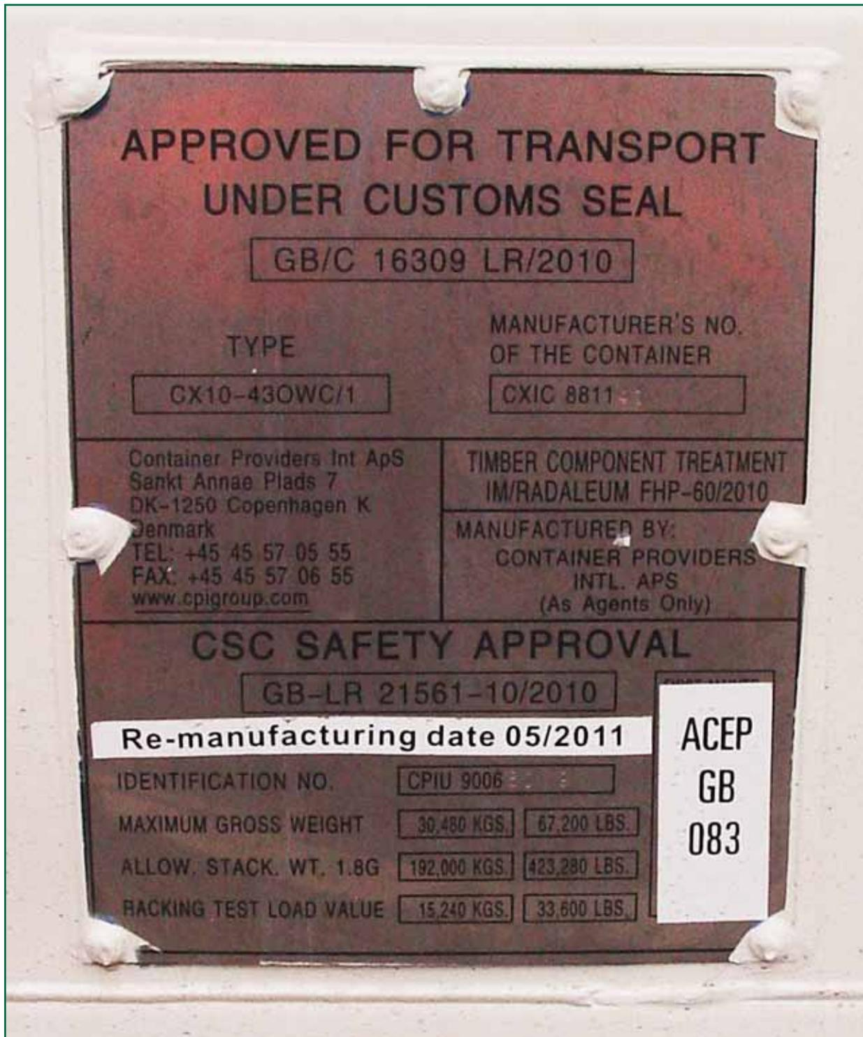
Figure 10: Safety approval plate fixed to container CPU 9006609. The RAIB understand that the white decal, entitled 'Re-manufacturing date 05/2011', was affixed when the container was modified (paragraph 20). Note: Recognised by the CSC as acceptable practice, the safety approval plate has been grouped with other official plates on one base plate
