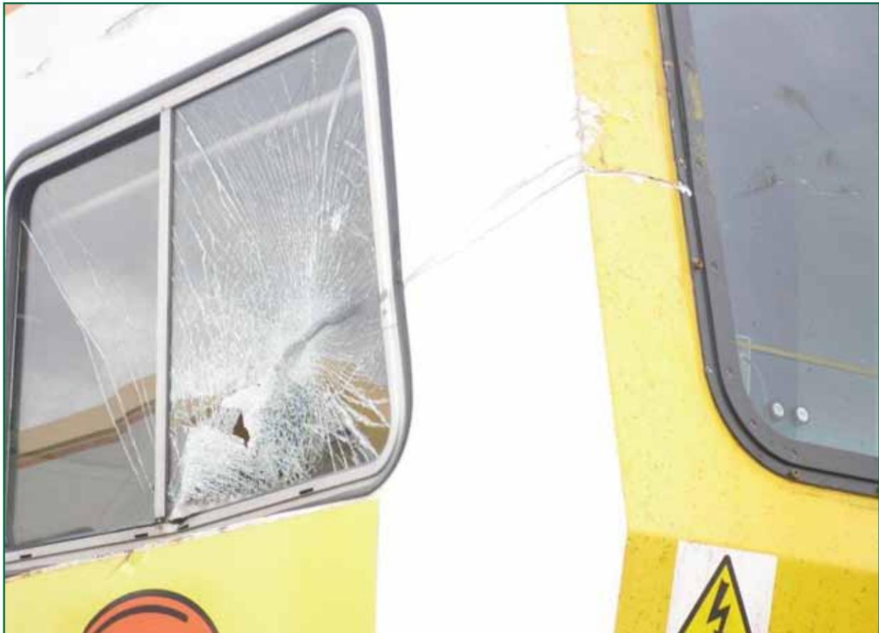
Figure 9: Damage done to the driving cab of the tamper (photograph courtesy of Colas Rail)
