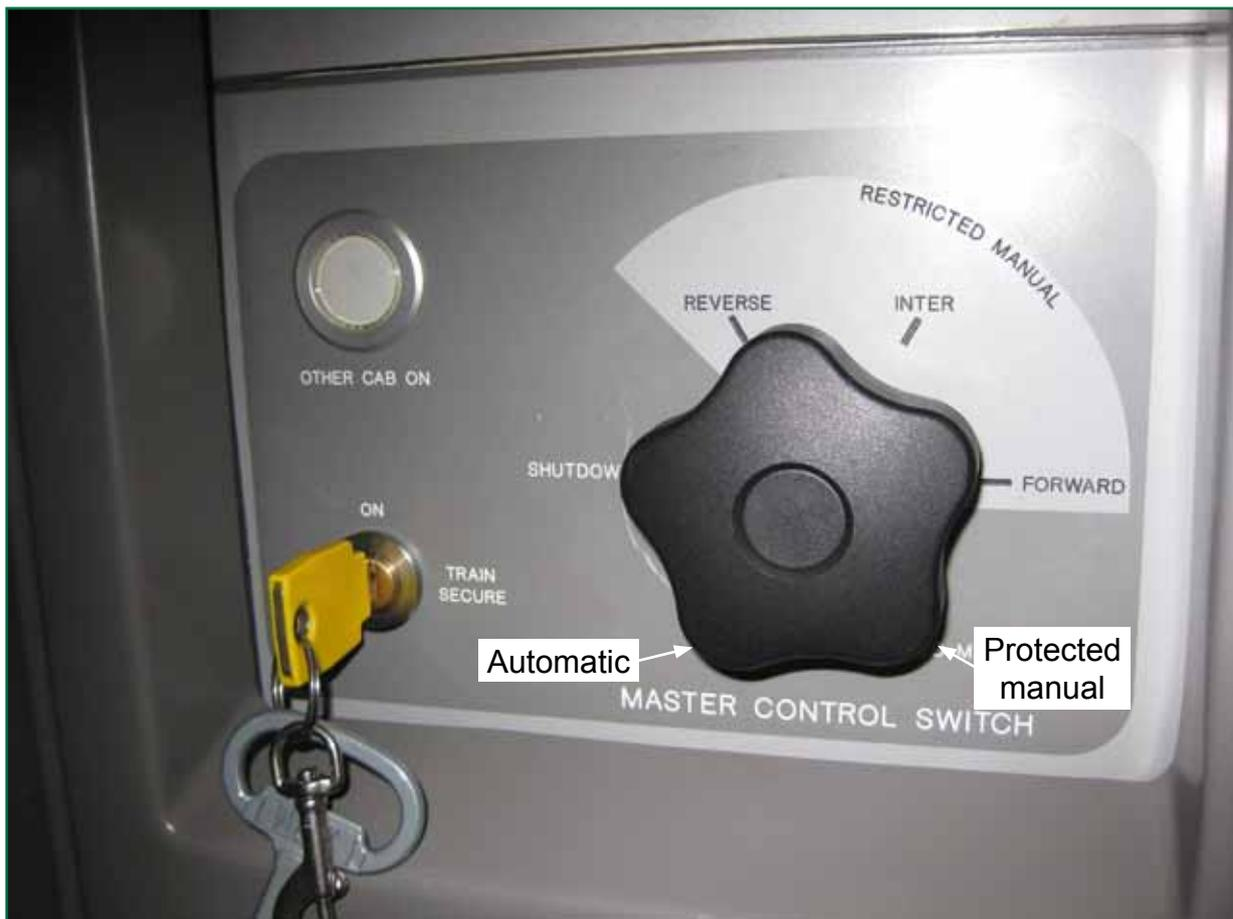
Figure 4: Master control switch 2009 tube stock
