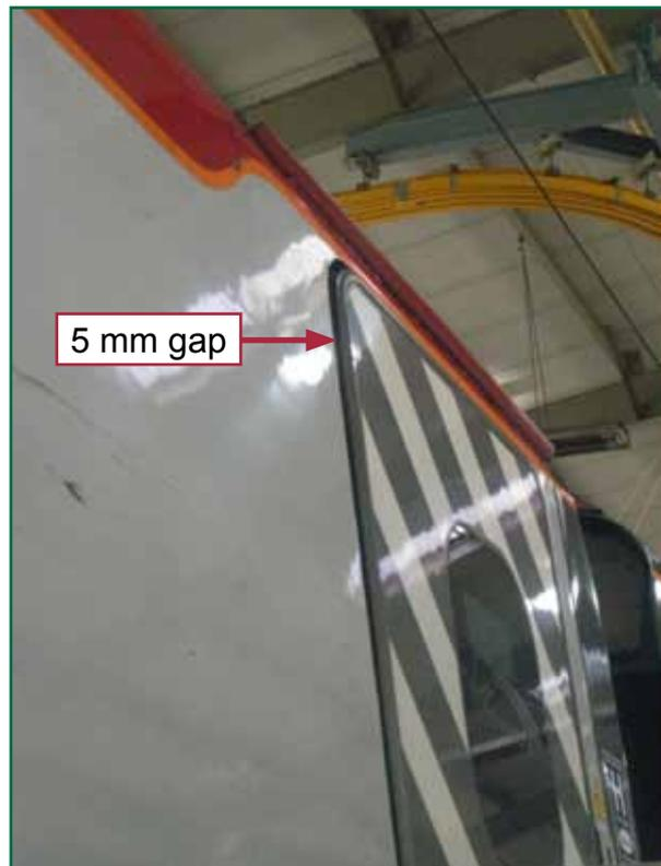
Figure 3: external view of door, locked out of use but not fully closed
