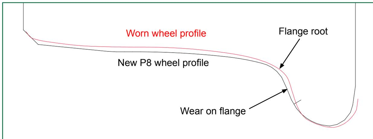
Figure 6: Wear to the flange thickness on first wheel to derail compared with new P8 wheel
