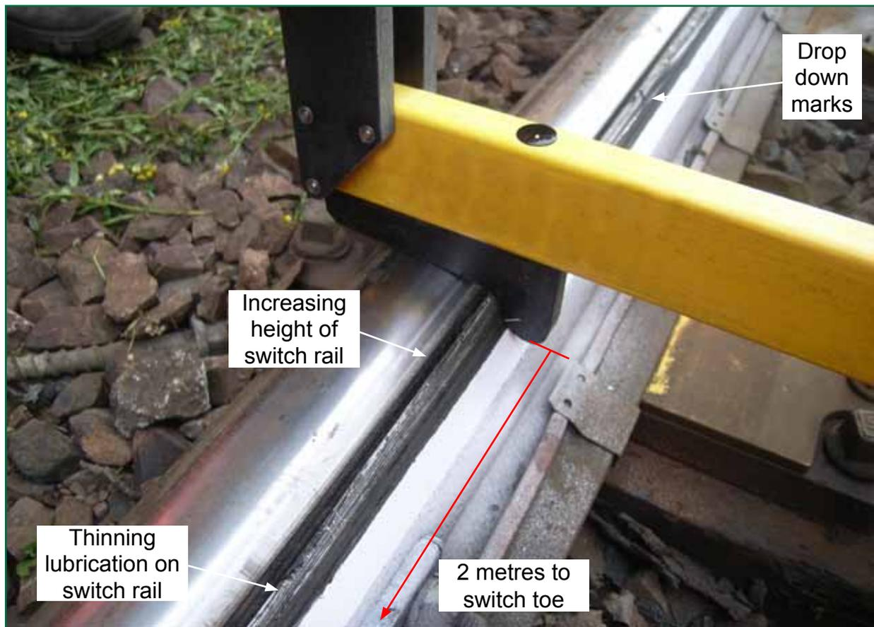
Figure 12: TGP8 gauge applied to left-hand switch rail of points 167B 2 metres from the switch toe
