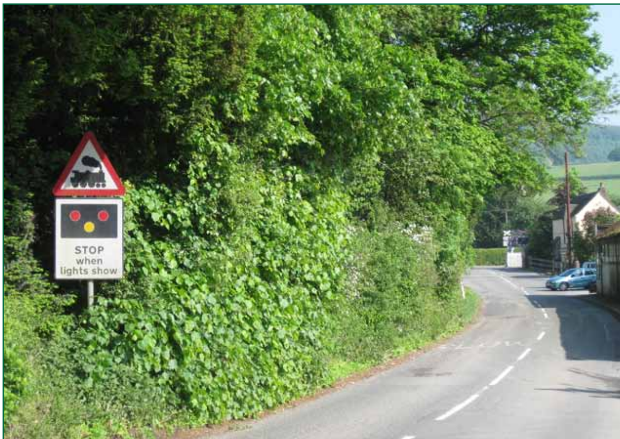
Figure 3: Road signage on the approach to an automatic open level crossing
