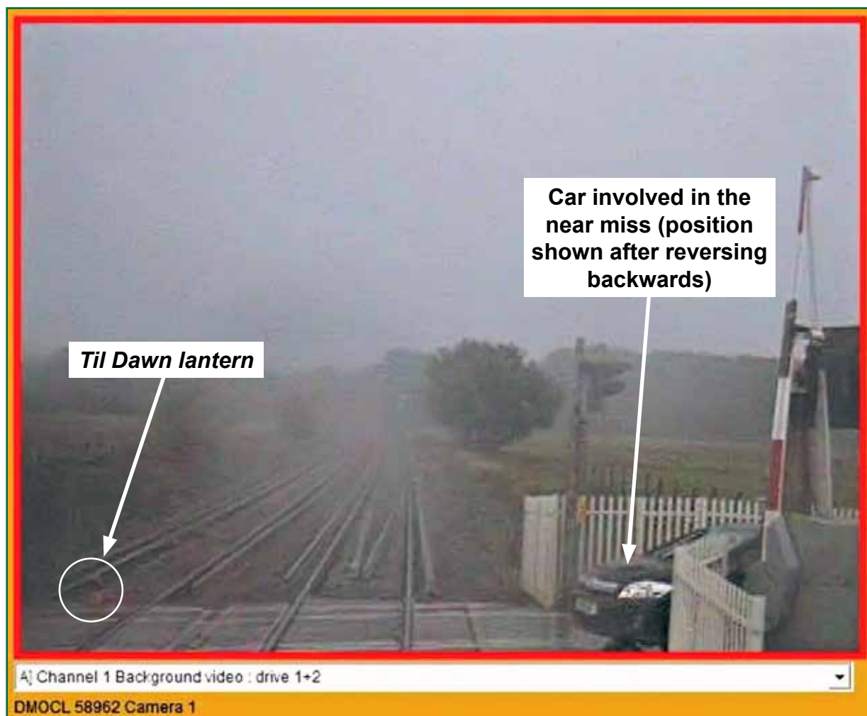
Figure 10: Rear facing CCTV image from train 1K54 showing Ufton Crossing and the car involved in the near miss
